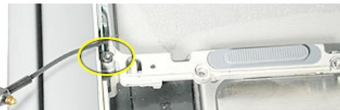
14. Lift the rib frame off of the heat exchanger. If the heat exchanger sticks to the rib frame, press gently on the heat exchanger near the two connection points shown.
