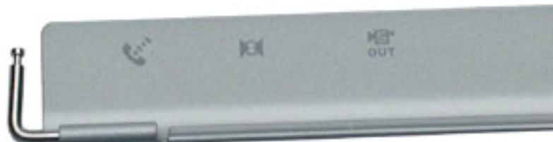
4. Install the replacement I/O door. Make sure each L-shaped pin threads through the top case, inner clutch mount, spring, and plug.
