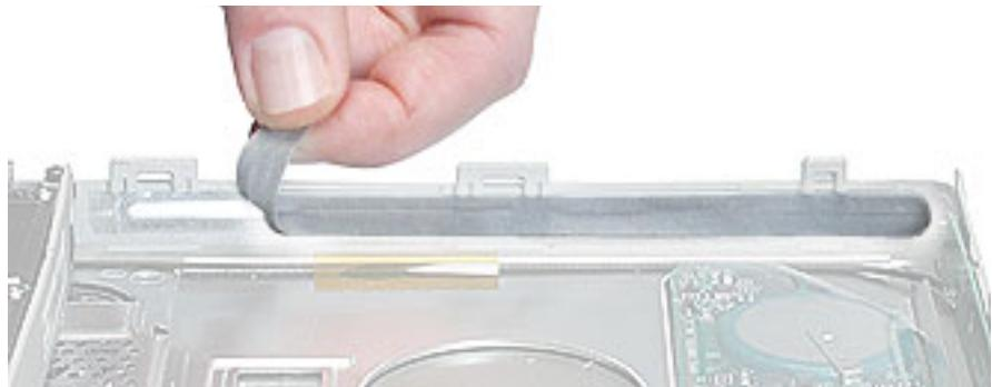
Apply the new felt strip to the slot-load area. Make sure the new felt strip lies flat. Use a black stick to run the length of the slot to make sure that the felt strip does not block any of the slot.
