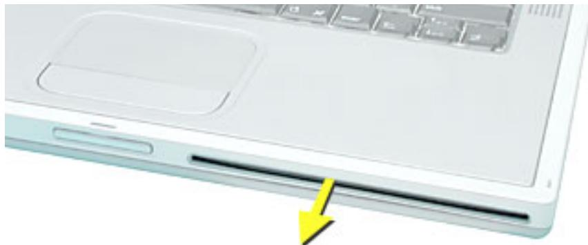
**Important:** Check the operation of the optical drive. If the drive is installed incorrectly, the optical drive mechanism might not spin correctly and will result in mechanical noise when playing a disc.
