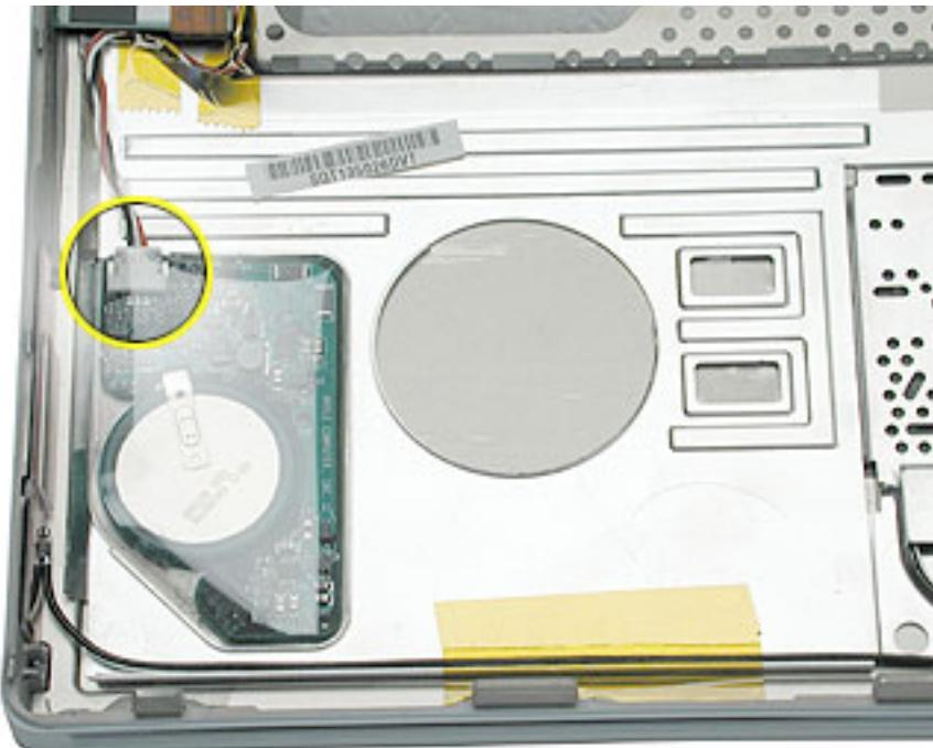
2. **Note:** The backup battery is compressed between two thin plastic sheets. The battery is held in place with adhesive on the lower plastic sheet.
