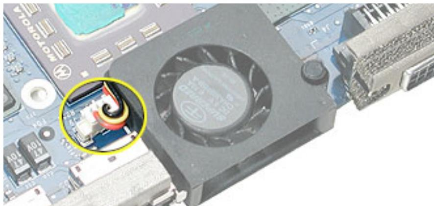
2. Turn over the logic board, and locate the cone-shaped pin at the right corner of the fan. Pull the rubber pin tight. Use a razor blade to cut through the rubber pin.
