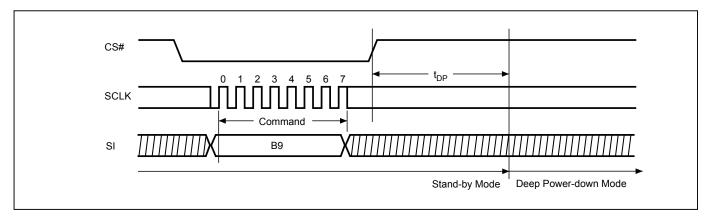
Figure 24. Release from Deep Power-down (RDP) Sequence (Command AB)
