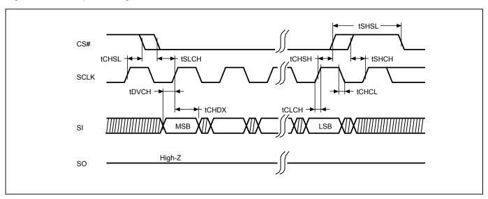
Figure 9. Output Timing
