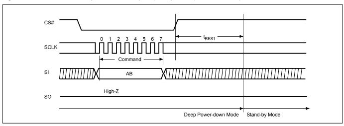
Figure 25. Read Electronic Signature (RES) Sequence (Command AB)
