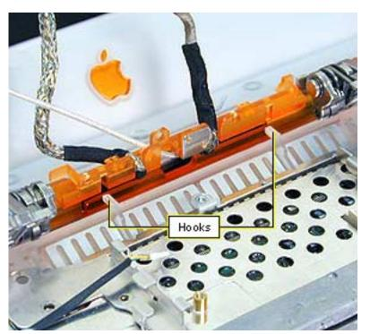
Move the display straight back to clear the two hooks near the center of the clutch.
