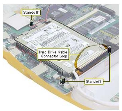
**Important:** Pull straight up to prevent bending pins on the logic board.
