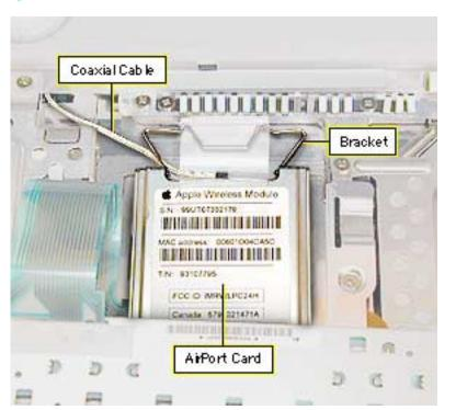
6 Flip up the wire bracket, and remove the installed AirPort Card from its connector. Disconnect the AirPort antenna coaxial cable.
