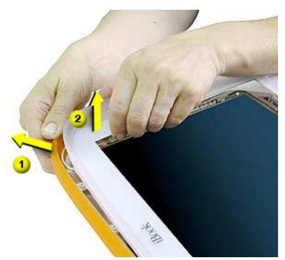
Work your hands around each side, separating the bezel from the display housing. At the top corners, pull the plastic of the display housing out while pulling up on the bezel.
