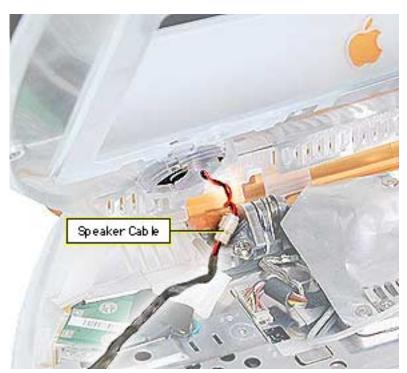
13. Carefully rotate the top case up and rest it against the display, then disconnect the speaker cable.
