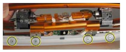
8. Remove the four exterior screws on the display housing.
