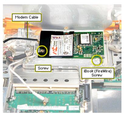
the large Phillips screw attached to the computer's framework near the right front edge of the modem.
