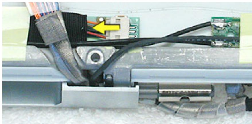
6. Remove the reed switch cable assembly.
