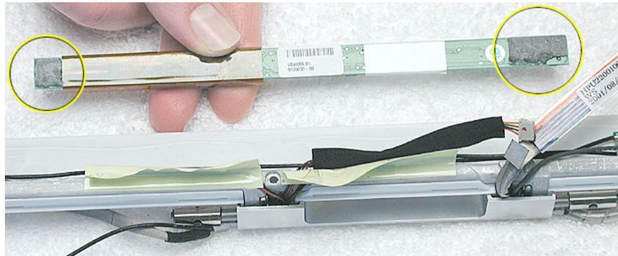
4. Install the replacement inverter board, and reassemble and test the computer.
