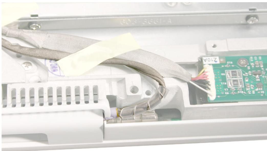
7. **Important:** Create enough slack in the cable near the connector to relieve tension on the cable. Secure the connector and cable with a strip of Kapton tape, as shown.
