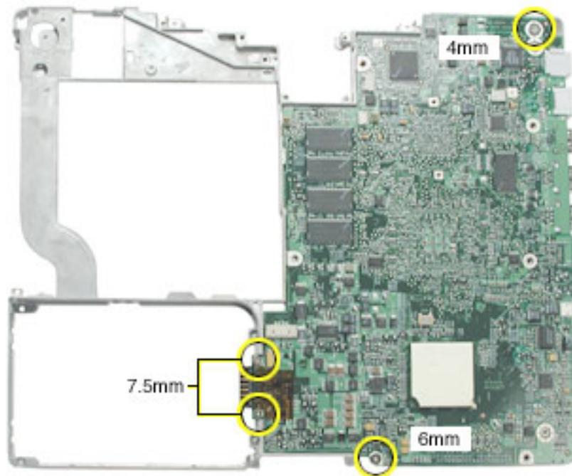
8. **Warning:** Flexing the logic board can break solder joints to components. To prevent damage, do not flex the board.
