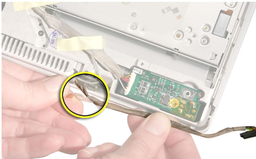
5. Make sure the tubing covers the cable where it exits the display.
