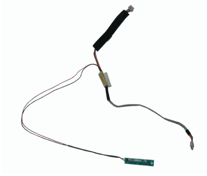
7. Install the replacement reed switch board and cable assembly, and reassemble and test the computer.
