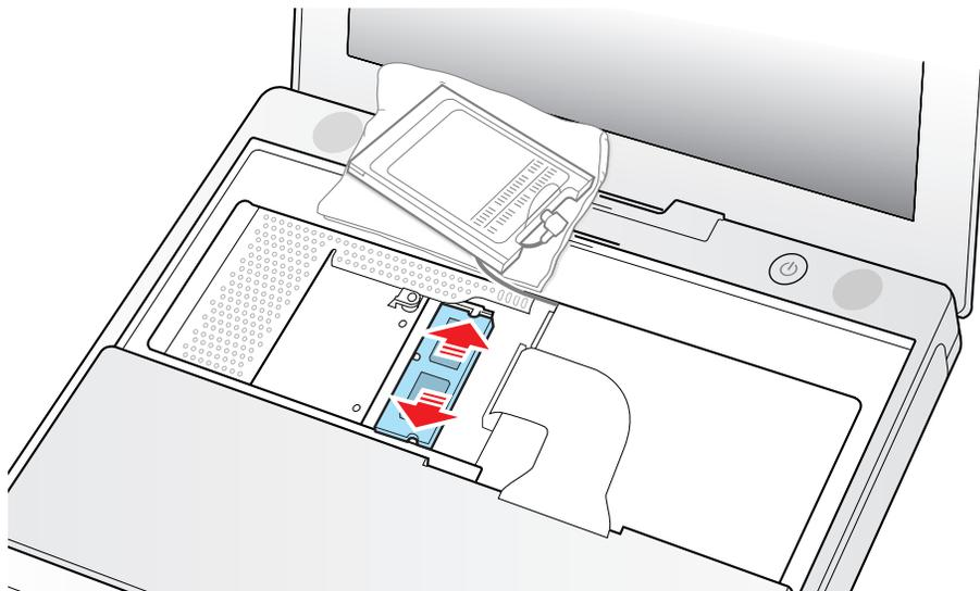
3. Line up the notch in the replacement memory card with the small tab in the memory slot. Hold the card at a 30-degree angle, then push the card into the slot until it is firmly seated.
