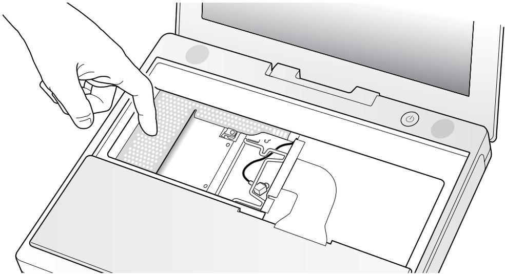
6. If the computer has the optional AirPort Card installed, unlatch the flexible wire holder that secures the card.
