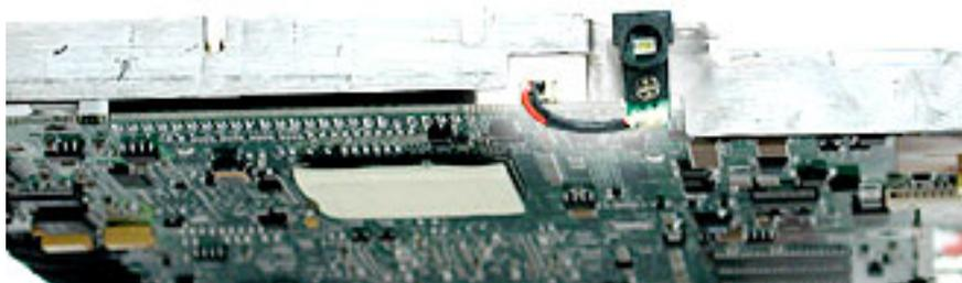
2. Using a black stick, disconnect the sleep light board connector from the logic board.
