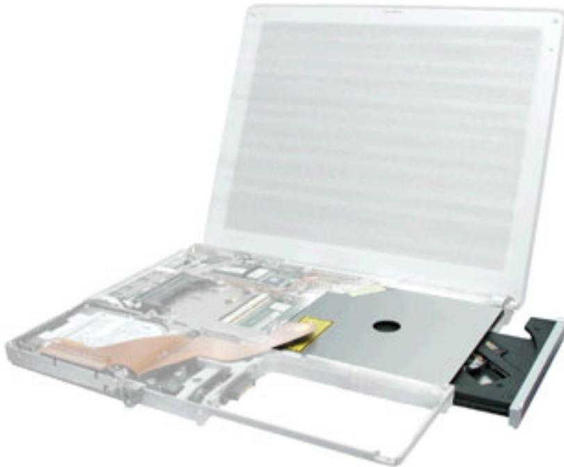
2. Tilt up the computer, and remove the two screws beneath the optical drive.
