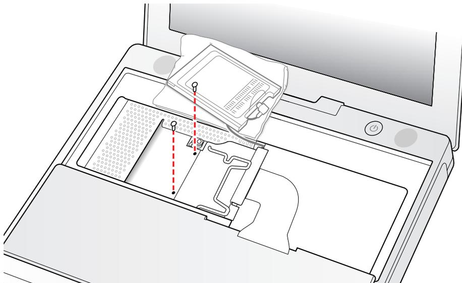
10. Lift the RAM shield out of the computer. Carefully pulling up on the wire holder may help to remove the shield.
