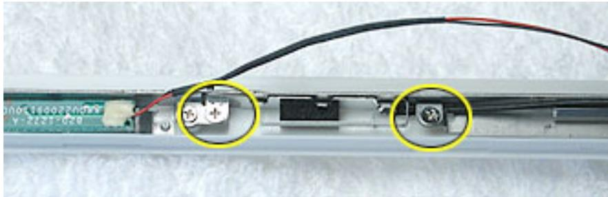
9. Tilt up the antenna receptor to remove it from the left side of the bezel assembly.
