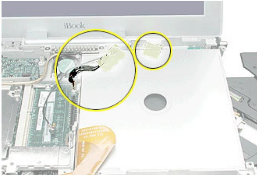
5. **Warning: Handle the optical drive at the sides only. Do not touch or press anywhere else on the drive.**
