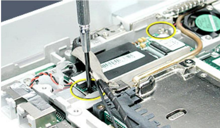
3. Tilt up the end of the modem to disconnect it from the logic board.
