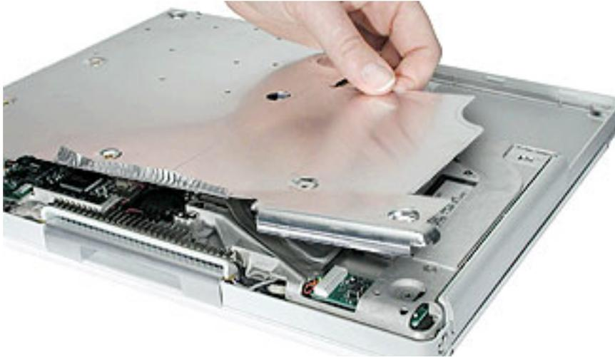
6. **Note:** The two springs in the battery connector can become loose. When reassembling the computer, make sure that the two springs in the battery connector are in place before installing the bottom case. Each spring might have grease on the coils, and each has a plastic cap on one end. Make sure the cap fits securely on the spring, and the curved side of the cap is positioned against the inner frame.
