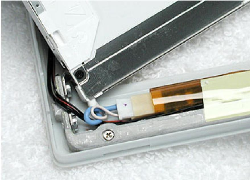
15. Install the replacement LCD panel, and reassemble and test the computer.
