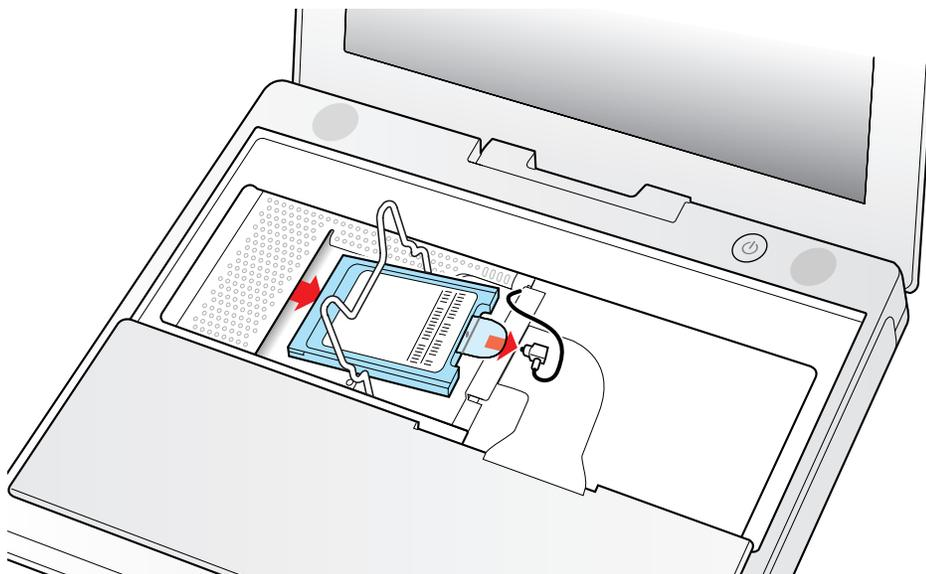
3. Use the pull-tab on the card to remove it from the slot.
