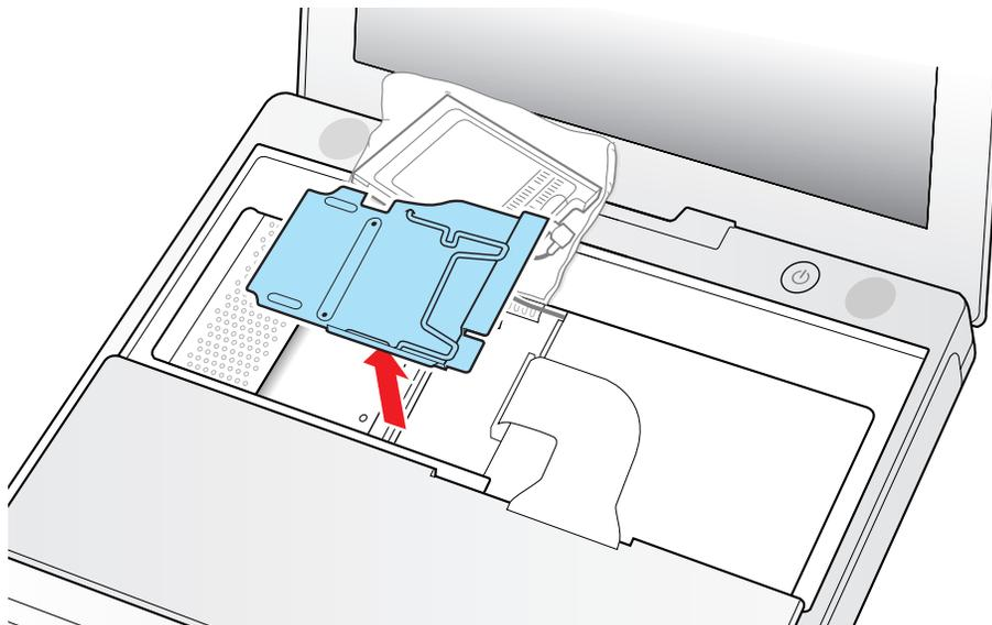
11. Locate the keyboard cable connector.
