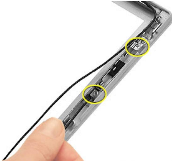
6. Tilt up the antenna receptor to remove it from the bezel assembly.
