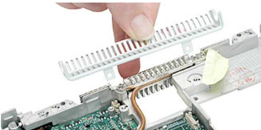
4. Turn over the computer frame and remove the two Phillips screws that secure the logic board to the heat spreader plate:
