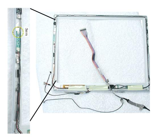
3. Lift up the cables and peel up the tape that covers the cables running along the bottom of the inverter board.
