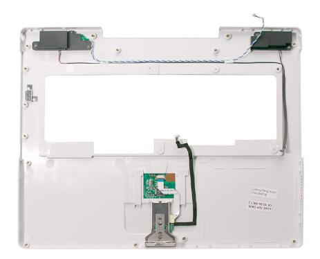
13. Install the replacement top case, and reassemble and test the computer.
