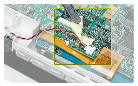
4. Turn over the computer and remove the single screw from the sleep light holder and frame.
