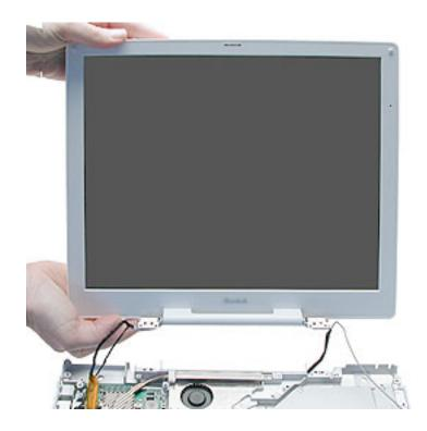
10. Install the replacement display module, and reassemble and test the computer.
