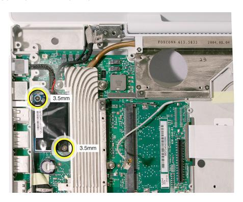
4. Use a black stick to lift up one end of the modem board. Grasp the top and bottom edges of the modem and metal shield to disconnect them from the computer.
