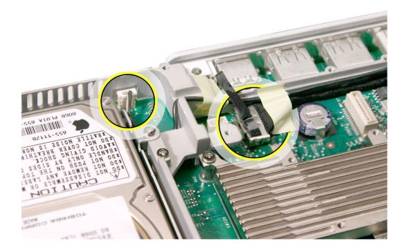
4. Carefully route the AirPort antenna cable out from under the optical drive.
