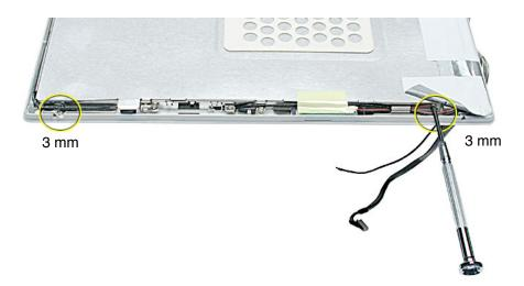
7. Peel up the foil tape that holds the LCD cable to the LCD shield.
