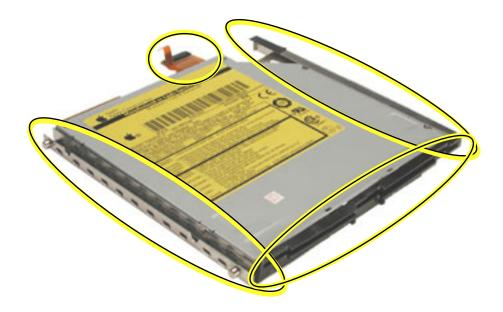
1. Remove the four identical screws that hold the top cover to the drive.
