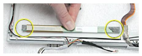
3. Install the replacement inverter board, and reassemble and test the computer.
