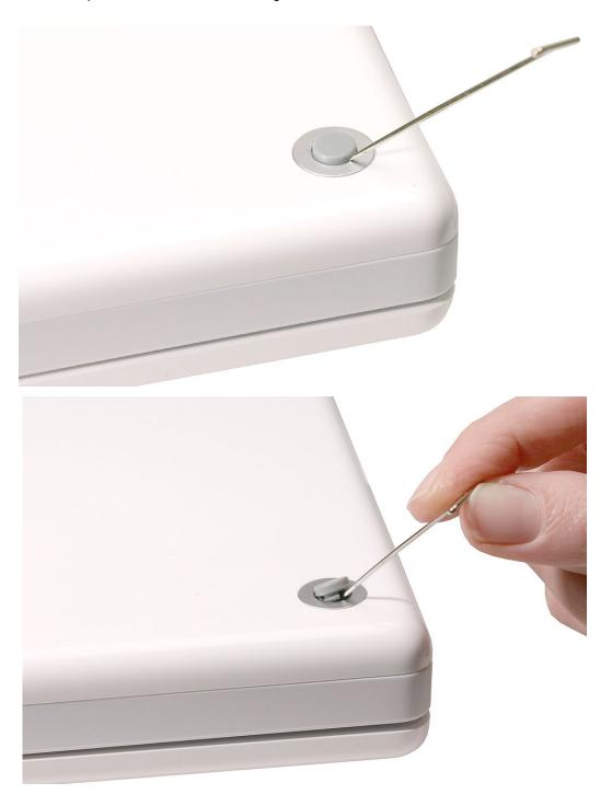
**Note:** If a portion of the rubber foot remains on the bottom case, use tweezers or needlenose pliers to carefully remove it.
