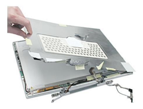
11. On the back of the LCD panel, grasp both sides of the LCD connector, and gently rock and pull the connector to disconnect the LCD cable from the LCD panel.
