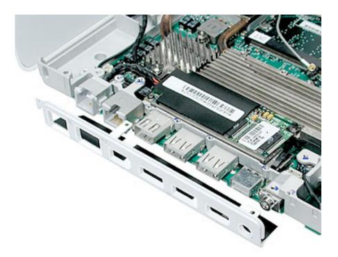
3. Install the replacement I/O bezel, and reassemble and test the computer.
