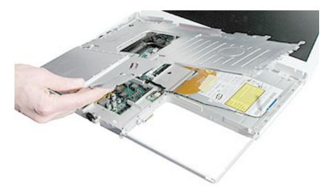
5. Install the replacement top shield, and reassemble and test the computer.
