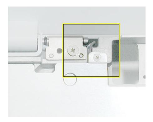
3. Carefully remove the Bluetooth antenna, if provided, from the top shield.
