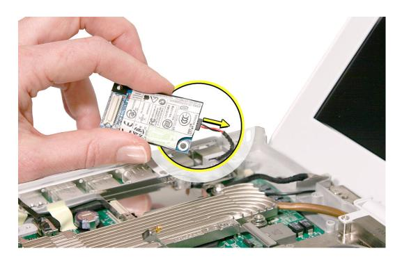
6. Install the replacement modem, and reassemble and test the computer.
