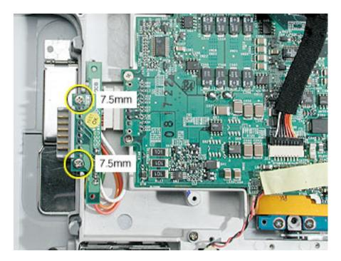
2. Disconnect the battery transfer board from the logic board.
