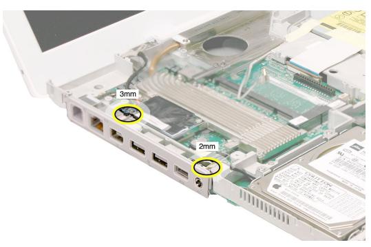
2. Remove the I/O bezel from the computer frame.
