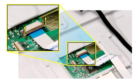
3. With the locking connector tilted up, slide out the trackpad cable.
