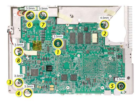
**Note:** When reassembling the computer, make sure that you transfer the following items from the original logic board to the top of the replacement logic board:
