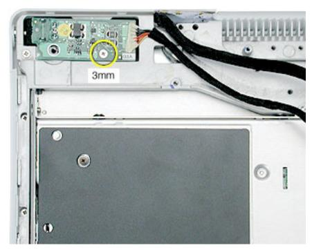
5. Tilt up the DC-in board, and pivot it out of the frame.
