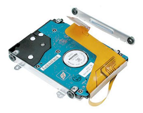
8. Warning: Handle the hard drive at the sides only. Do not touch or press anywhere else on the drive.
