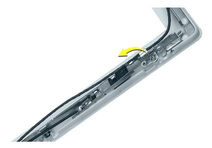
9. On the left side of the bezel, remove the two Phillips screws at the antenna receptor.
