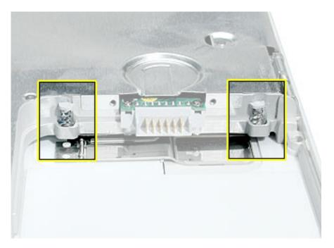
**Note:** When reassembling the computer, make sure that the two springs in the battery compartment are in place before installing the bottom case. Each spring has a plastic cap on one end. The cap should fit securely on the spring, and the curved side of the cap should be positioned against the inner frame. The springs have a small amount of grease on them; do not wipe away the grease.
