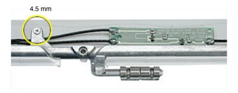
5. Lift up the bezel brace and release the cables from under the brace.
