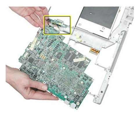
6. Install the replacement logic board, and reassemble and test the computer.
