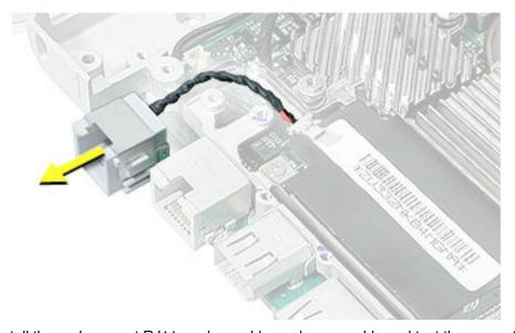
4. Install the replacement RJ11 modem cable, and reassemble and test the computer.
