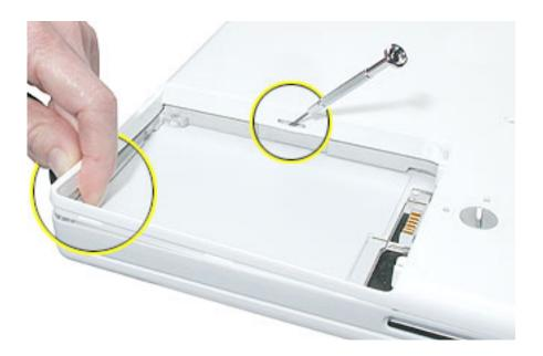
13. Loosen the tabs from the slot load area last.
