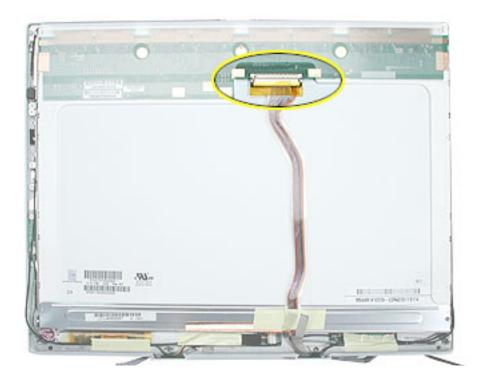
12. At the other end of the LCD cable, remove the tape from the bottom edge of the LCD panel.
