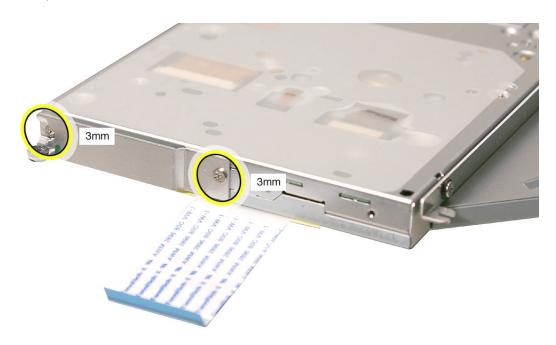
8. Peel off the tape from the optical drive, and disconnect the ribbon cable.
