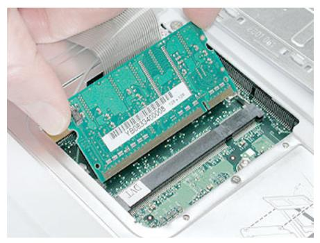
5. Gently push the top of the card down until the brackets snap onto both sides of the memory card to lock it into place.
