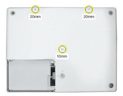
3. Using a pin, pry up the three rubber feet from the metal sockets.
