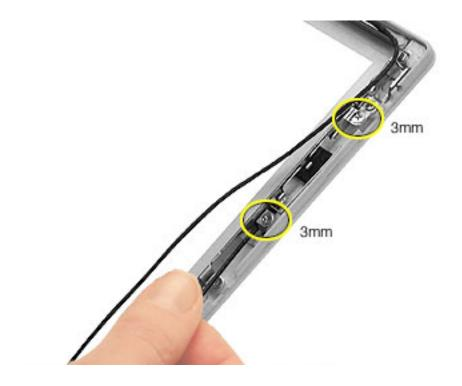
8. Tilt up the antenna receptor to remove it from the bezel assembly.
