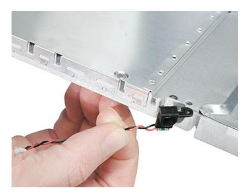
6. Install the replacement sleep light board, and reassemble and test the computer.
