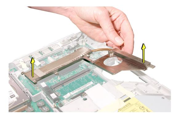
3. Turn over the heatsink and note the placement of the thermal pads.
