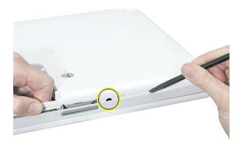
10. Open the computer and place it on its side. Carefully work the black stick around the corners of the bottom case.
