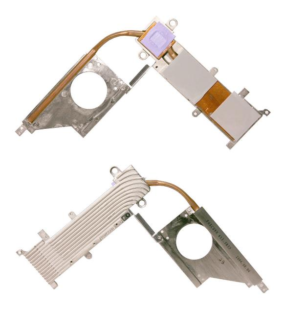
**Replacement Note:** If the thermal pads remain on the logic board, carefully remove them with a black stick. Check for any thermal pad residue remaining on the chips.
