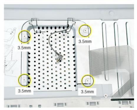
**Replacement Note:** Note the routing of the AirPort antenna cable. When reinstalling the RAM shield, make sure the antenna cable is routed as shown if there is no AirPort Extreme Card.
