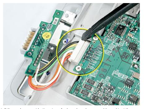
3. Install the replacement battery transfer board, and reassemble and test the computer.
