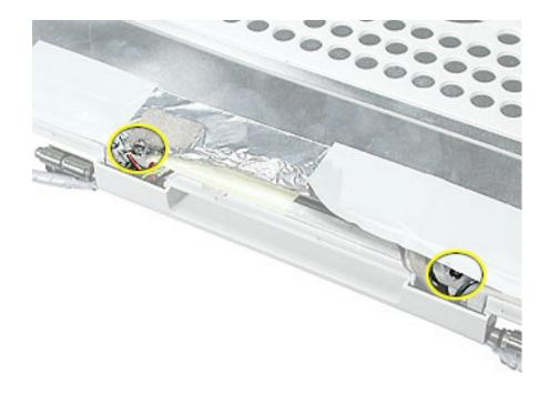
6. Tilt up the display assembly and pull straight down on the display clutch cover.
