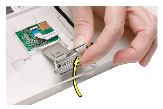
5. Carefully peel up the trackpad cable from the top case.
