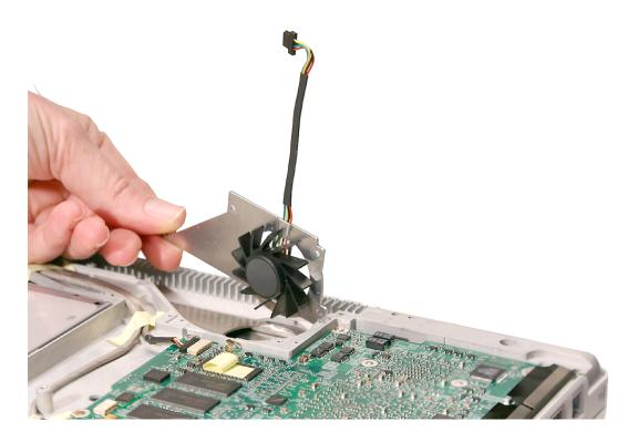
5. Install the replacement fan, and reassemble and test the computer.
