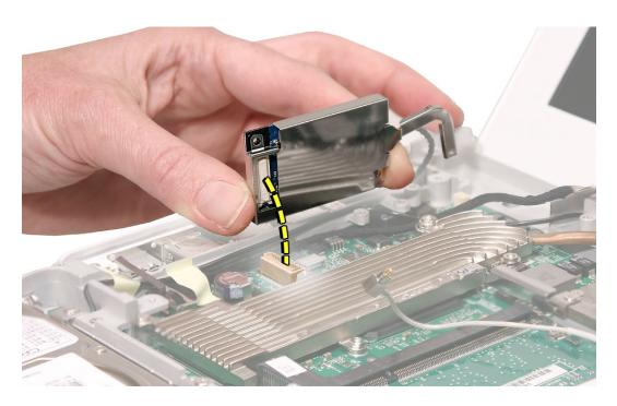
5. Disconnect the cable from the end of the modem board.
