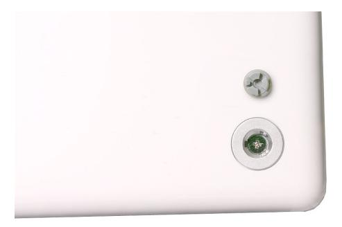
6. Remove the two identical Phillips screws next to the battery connector.
