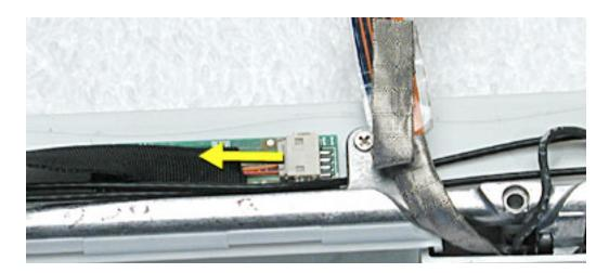
6. Remove the reed switch cable assembly.
