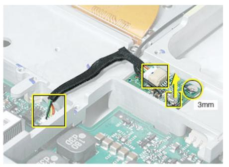
4. Install the replacement Bluetooth board and antenna, and reassemble and test the computer.
