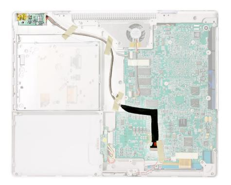
4. Remove the screw from the DC-in board.
