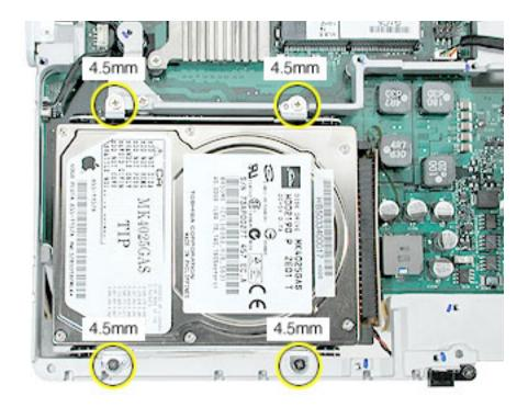
From the bracket side, tilt up the hard drive, and hold it by the sides of the drive.
