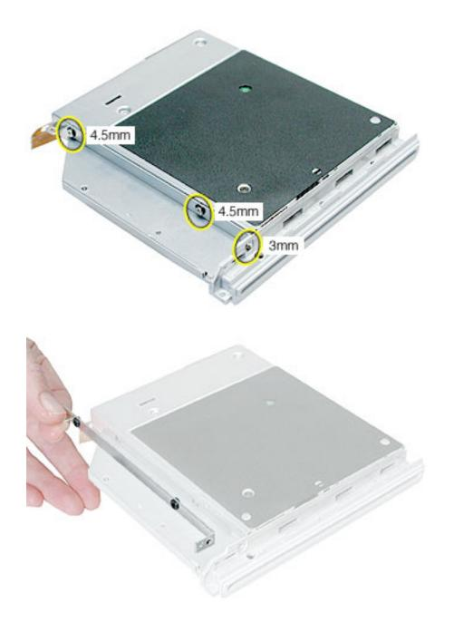
11. With the pointed end of a black stick, press the three tabs, and tilt the bezel up and off of the drive.
