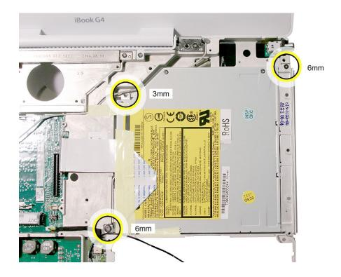
4. Disconnect the optical drive ribbon cable from the logic board.
