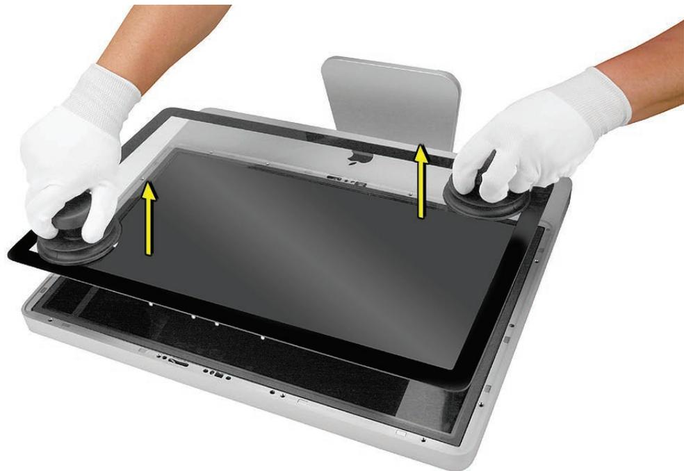
6. Set the glass down on the microfoam bag or clean lint-free surface and remove the suction cups. Squeeze the base of each suction cup to release them from the glass panel.
