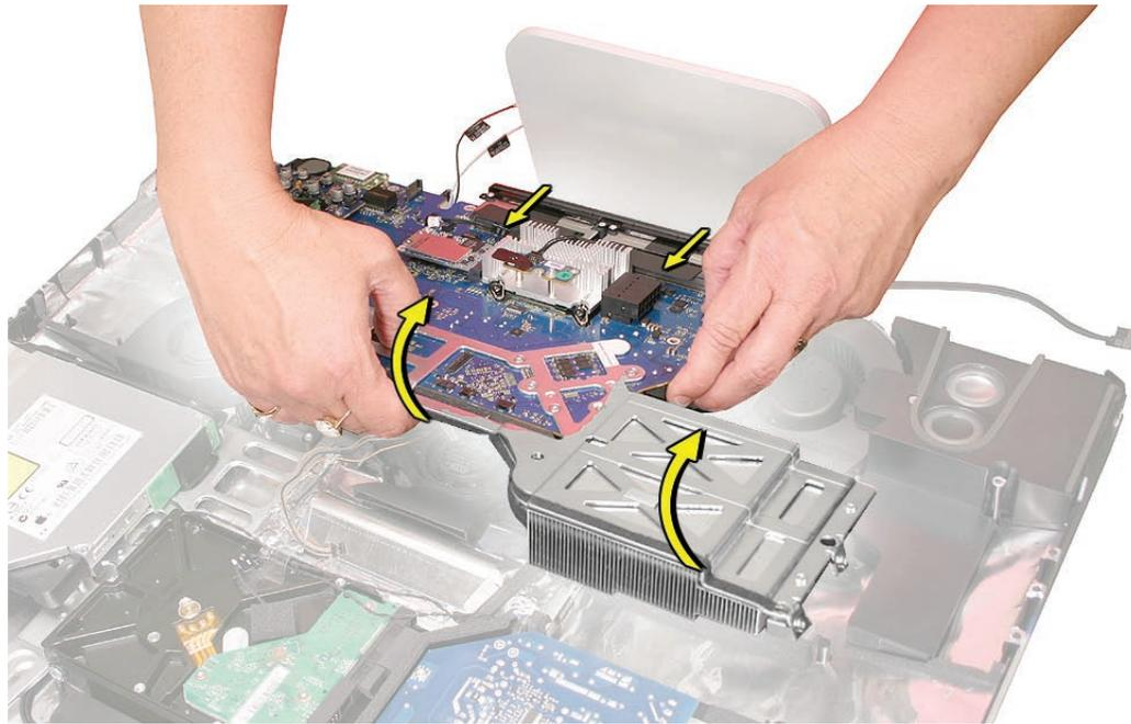
7. Transfer the video card on the back of the logic board to the replacement logic board.
