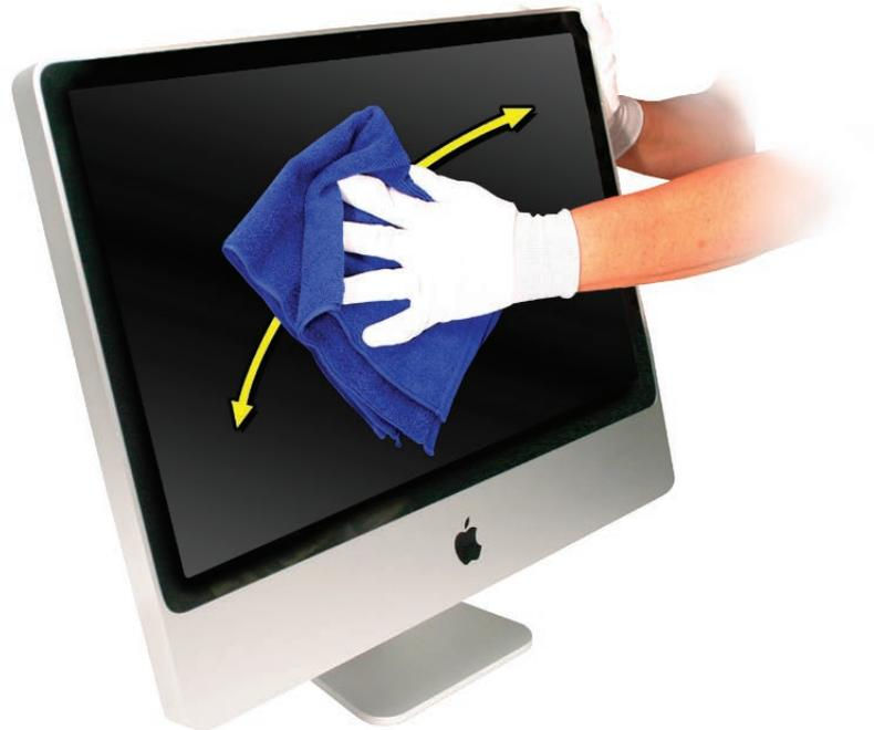
9. Once the glass has been cleaned and polished, visually inspect the glass for any remaining dust, fingerprints, or a hazy residue. If there are contaminants trapped between the LCD panel and the glass panel repeat the cleaning procedure described in this section before returning the system to the customer.
