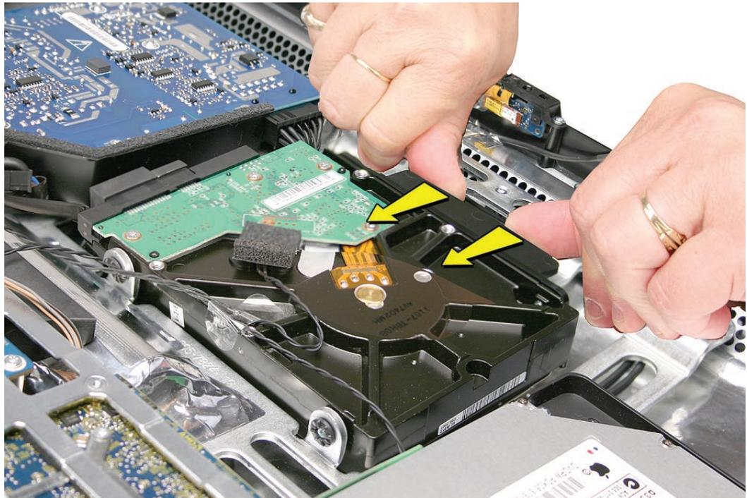
3. Disconnect the power and data cables from right side of the hard drive.
