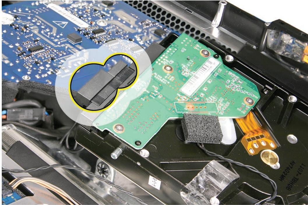
4. Lift the hard drive from the computer assembly.
