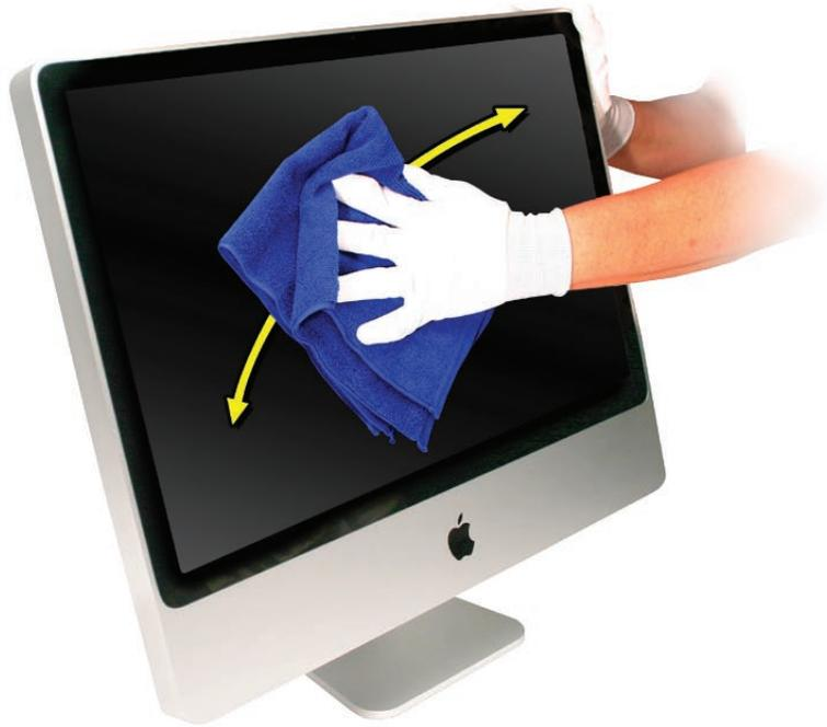
14. Once the glass has been cleaned and polished, visually inspect the glass for any remaining dust, fingerprints, or a hazy residue. If there are contaminants trapped between the LCD panel and the glass panel repeat the cleaning procedure described in this section before returning the system to the customer.
