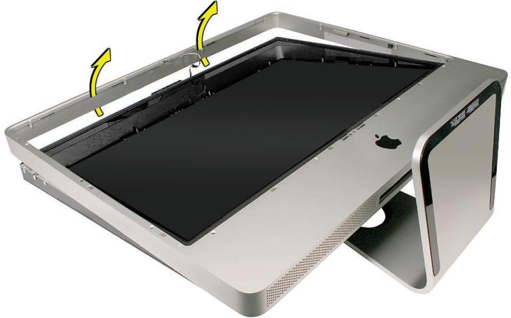
5. Notice the connected microphone cable at the top of the bezel. Without straining the cable, hold the bezel up, and disconnect the microphone cable from the cable extension.
