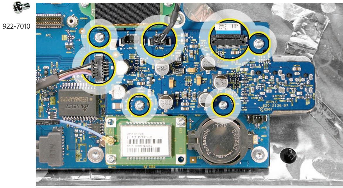
3. Replace the right speaker and connect the speaker cable to the audio board.
