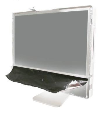
4. Using the access tool, a black stick, or your fingers, peel the black EMI tape off the right and left sides of the panel.
