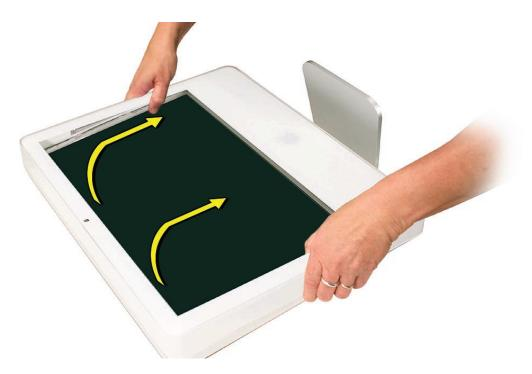
10. Swing the bezel up so you can disconnect two cables on the camera board at the top of the bezel.
