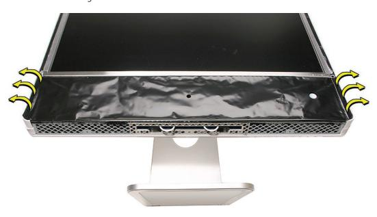
Peel the bottom of the EMI shield off the frame.
