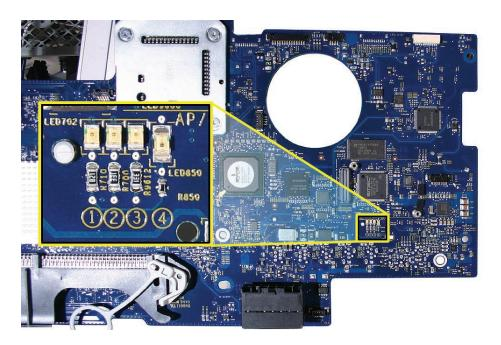
LED #1 is On: This indicates that the AC power inlet and AC-to-DC power supply is getting good power from the AC outlet, and the DC-to-DC board is receiving 12VDC. Go to step 8.
