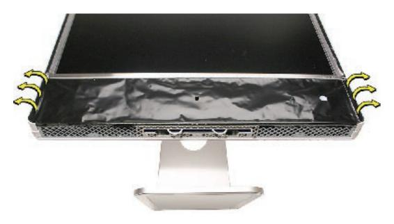
2. Carefully peel the lower EMI shield off the bottom edge of the rear housing. Use a black stick to help peel back the shield.
