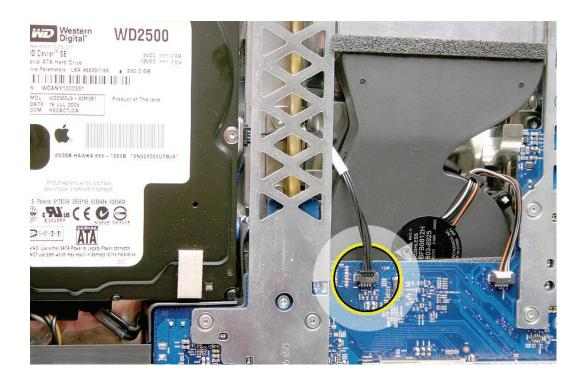
Insert the hard drive pins into the grommets. Lower the drive into the rear housing.
