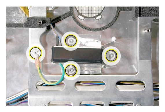
2. Carefully peel up the EMI tape on the AC filter; peel off both the large and small EMI pieces of tape. Set them aside.
