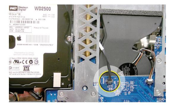
3. The hard drive sensor is different from the optical drive sensor. The hard drive sensor can be identified by resistor R1700. Replacement Note: Make sure to transfer the sensor to the replacement hard drive. Use the double-stick tape enclosed with the replacement hard drive to attach the sensor.
