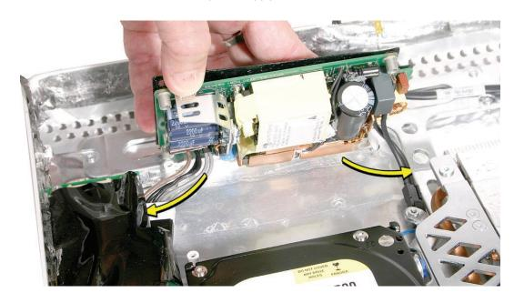
Replace the power supply screws. Install the machine screw (bottom right corner) first when installing the power supply.
