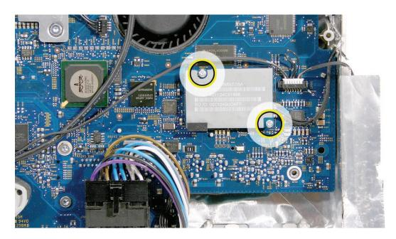
2. Disconnect the two antenna cables from the AirPort Extreme/Bluetooth card.
