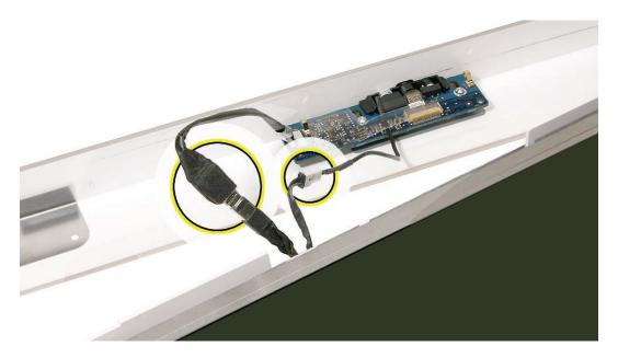
3. Tuck the cables neatly into the channel on the rear housing.
