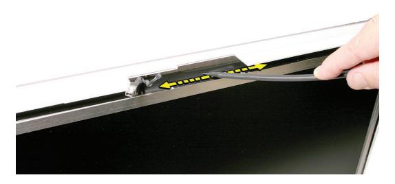
2. Connect the camera and microphone cables (on the camera board) to the cables sticking out of the top of the computer.
