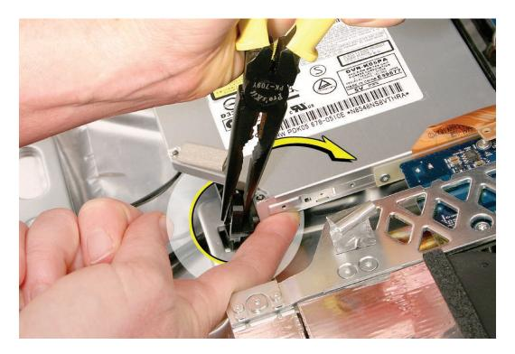
Caution: Never press down on or grasp the body (silver) of the optical drive when removing or installing it. Depressing the body of the optical drive could damage the mechanism. Grasp the optical drive by its mounting bracket only.
