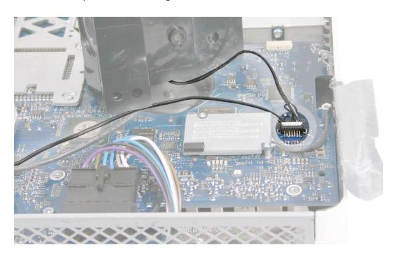
2. Install the speakers and route the speaker wire as shown below.
