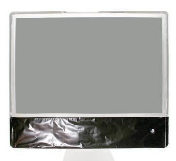
When properly repaired, all edges shown below will be wrapped by EMI tape, and the tape securely adhered to all edges. Use a "black stick" to flatten the EMI tape tightly and rub out air pockets and wrinkles.
