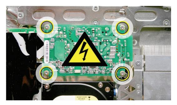
2. Lift the power supply up and remove the cable and connector from under the chassis. This cable connects to the AC filter board located under the logic board. Note the routing of the cable under the chassis.
