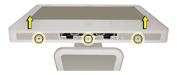
6. Stand up the unit. Using the plastic access card, unhook the bezel locking mechanism in one upper corner of the front bezel, and pull the bezel slightly away from the rear housing. Note: You must Insert the access card through the vent in the rear housing as shown below, and push it up and back until the latch releases.
