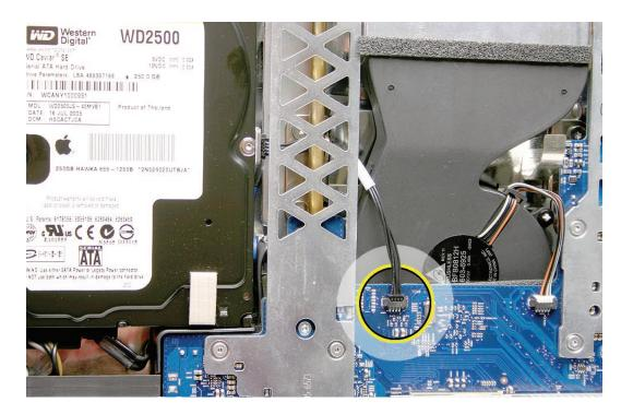
Replace the optical drive sensor cable, flex cable and screws, and the silver EMI tape.
