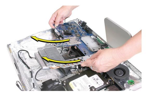
9. When handling the logic board, hold the board as shown below. **Important**: Never handle or carry the board by the heatsink or metal rails.
