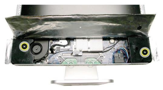
2. Using a T6 torx screwdriver, remove the screw that secures the IR board to the IR mounting bracket. Disconnect the IR cable from the IR board.
