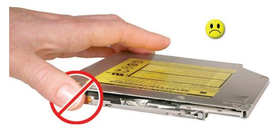
Do not press on the drive or lift it by the top and bottom cover.
