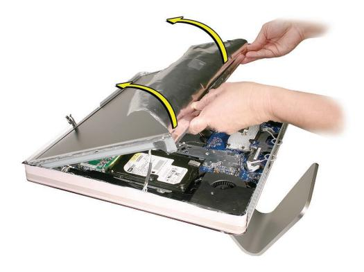
9. Disconnect the two panel-to-inverter cables on the bottom left side of the display. Replacement Note: The cable connectors are marked with dots to indicate "right-side-up".
