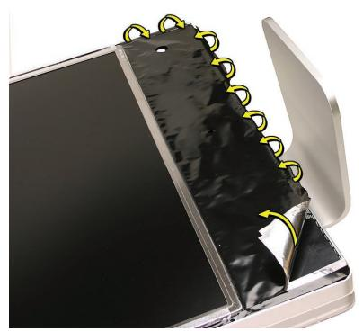
3. Peel the EMI housing up as shown.
