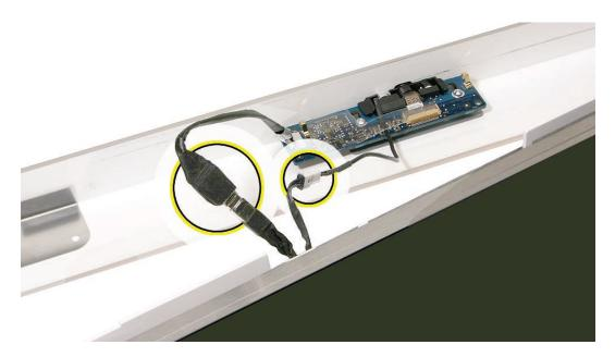
4. Tuck the camera board cables neatly into the channel on the rear housing.
