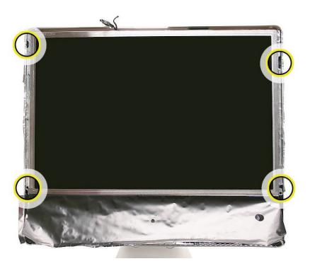
8. Lift the panel up just enough to see the inverter cables on the left side.
