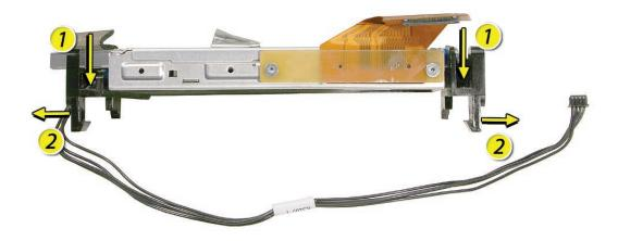
6. If replacing the optical drive, use a T6 torx screwdriver to remove two flex cable screws attaching to the optical drive. Note: Disconnect the flex cable and transfer it to the replacement drive. Go on to the next step.
