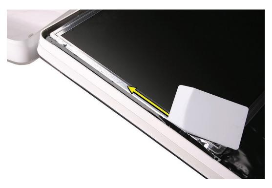
5. Using the access tool or black stick, peel back the black EMI tape stuck along the entire length of the top panel.
