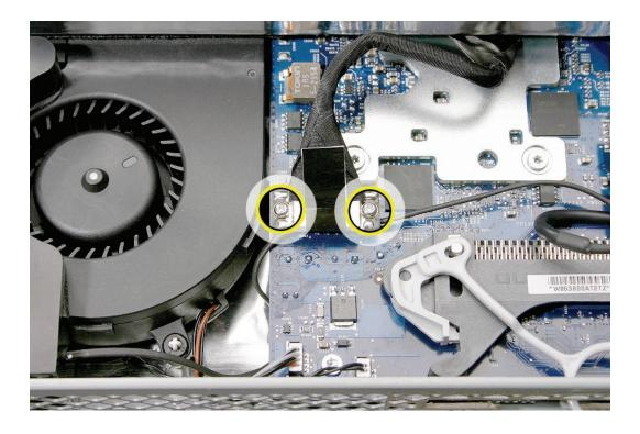
Using a Torx T10 screwdriver, remove the four panel mounting screws.
