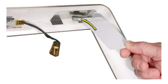
5. Start on the left side (looking from the back of the unit). As you insert the card to disengage the latch, squeeze the top of the bezel, that will help take pressure off of the latch and enable it to open easier. As the bezel releases, pull the bezel away from the rear housing.
