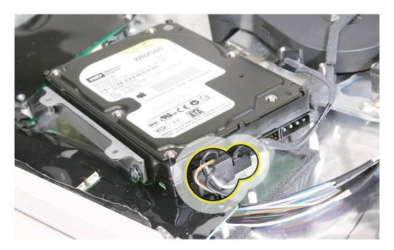
6. If you are replacing the hard drive, remove the temperature sensor, mounting bracket, and mounting pins (circled) before returning the drive to Apple. Transfer these parts to the replacement drive.
