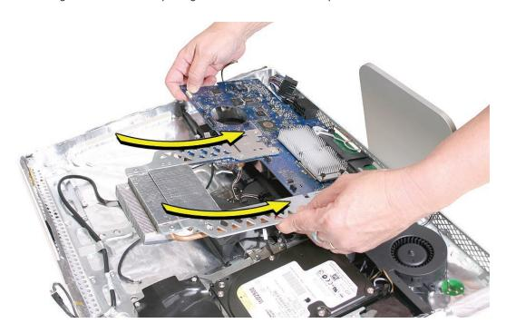
3. **Note:** If the replacement logic board doesn't have the support brackets (shown below) installed on the heatsink, transfer the brackets from the old board. Replace the two T6 screws on the top of the brackets and the T7 screws from the side support bracket.
