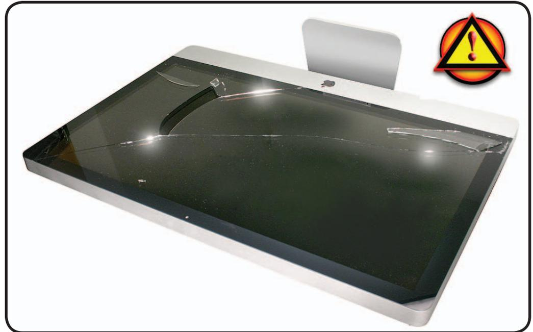
3. Peel protective covering off the front of the glass. Remove and discard any large pieces of broken glass.
