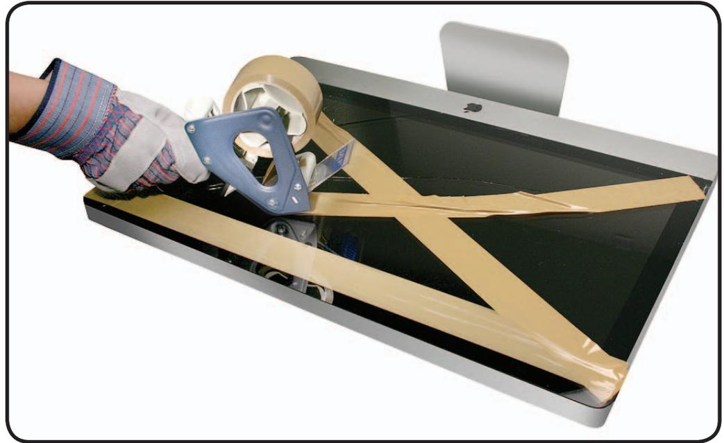
5. Continue applying tape horizontally, thoroughly covering the broken glass. Most of the glass will still be attached to the steel ring that runs around the perimeter of the glass panel.
