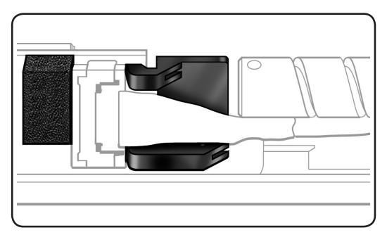
4 Disconnect 2 AirPort antenna cables using a black stick.
