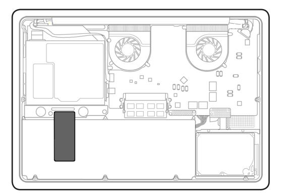
4 Without pulling cable, tilt out battery.
