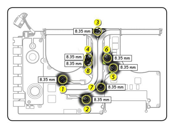
**3** Keeping heatsink parallel to logic board, gently wiggle the heatsink to loosen the bond to the board.
