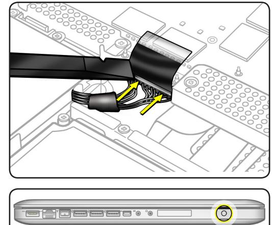
5 Press battery indicator light to check charge level.
