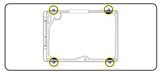
**3** Attach connector, and tilt hard drive into front of top case.
