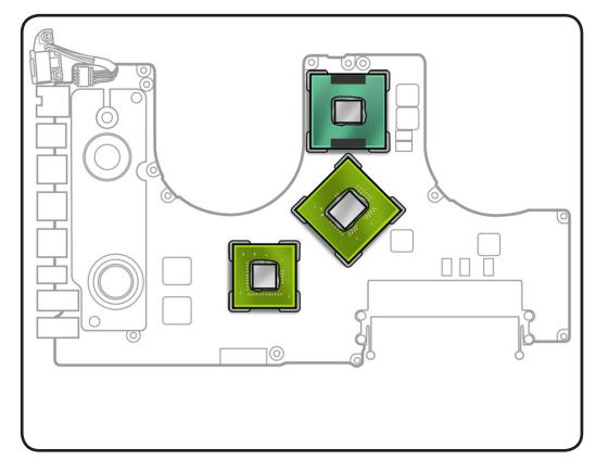
5 Install heatsink screws in order, 1/2 way first, then tighten the rest of the way.
