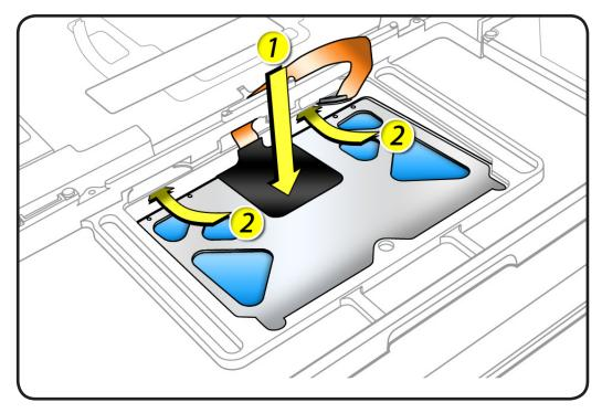
**9** Tilt up top case, and spiral trackpad away from top case while carefully routing flex cable through hole.
