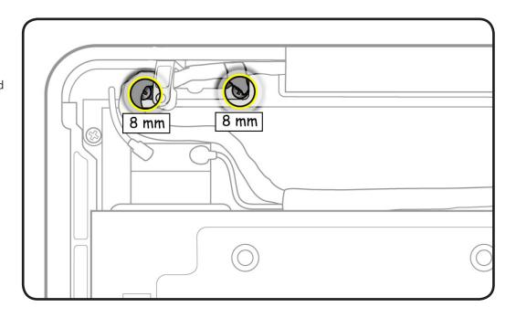
2 Remove the camera cable guide.
