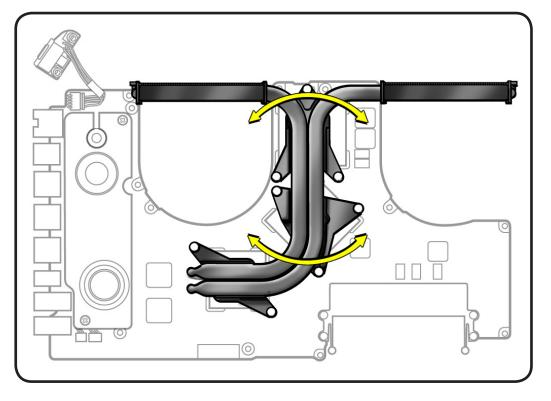
4 With a black stick, scrape off thermal grease and use alcohol pad to clean thermal pads and chips.
