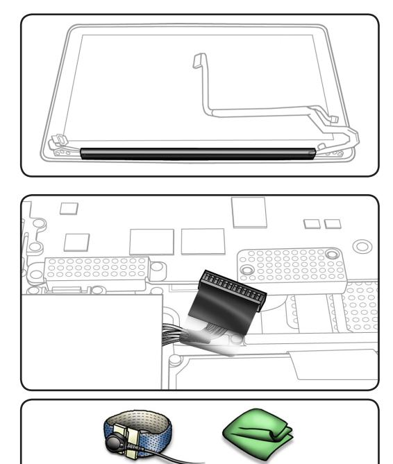
Before you begin this procedure, disconnect the battery from the logic board. Failure to do so could damage the computer.
