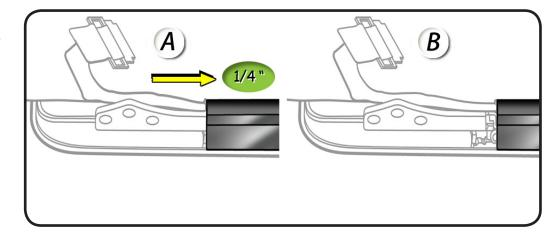
**3** Press down on clutch cover to loosen 4 hooks inside.
