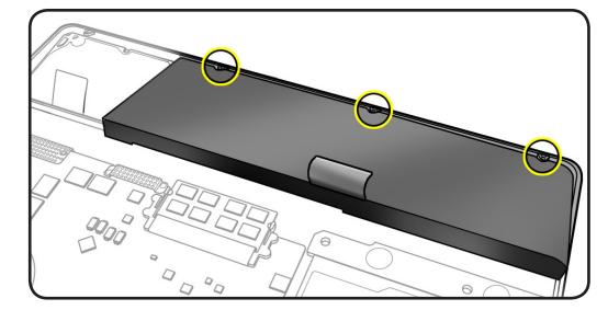
**3** If performing other repairs, be sure to leave battery cable disconnected.
