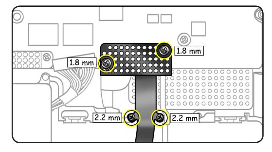
**3** Use black stick to disconnect cable and carefully pry cable up from adhesive.
