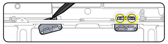
**3** Slide stiffeners over the flexures and align the screw holes.
