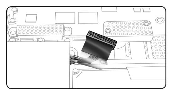
4 Connect battery cable using black stick or pull-tab, apply new battery label, and reassemble computer.
