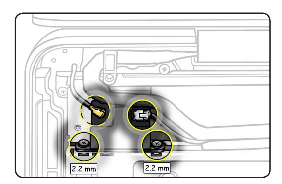
**3** Use black stick to pry out Bluetooth holder. (+) 3 + 4 Remove Bluetooth card and holder. 5 Turn over holder, and remove 2.3-mm screw 2.3 mm (part of 076-1348 kit) from metal bracket. **6** Lift out card from holder.
