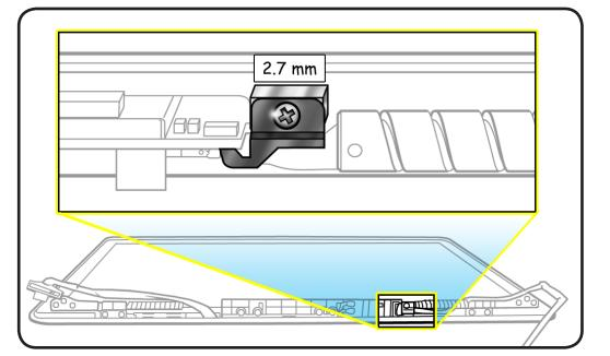
**3** Disconnect AirPort cable and remove cable clip.
