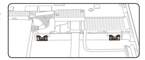
2 Make sure 4 Torx T6 (922-xxxx) mounting screws are installed on drive.
