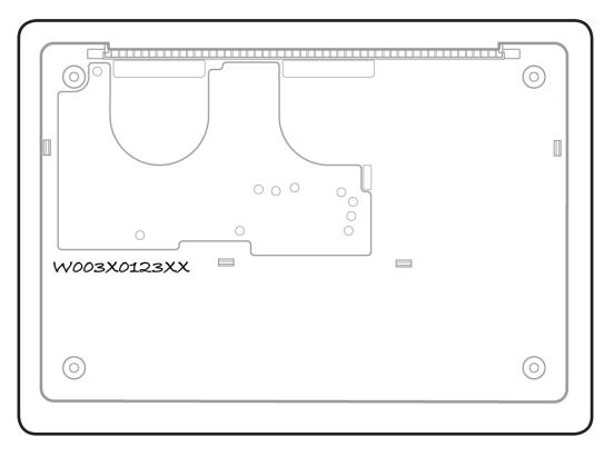
2 Install bottom case so that 4 clips snap onto top case.
