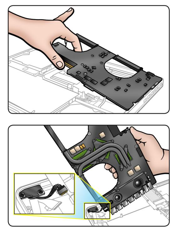
6 Holding board by edges, tilt it up and disconnect MagSafe connector.
