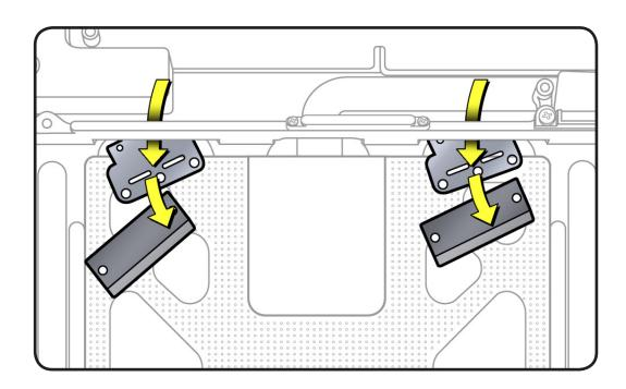
6 Carefully tilt up keyboard mylar as you peel up trackpad flex cable from adhesive on mounting ramp.
