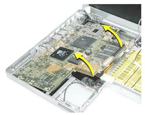
3. While holding the board vertically, disconnect the DC-in connector cable from the underside of the logic board.
