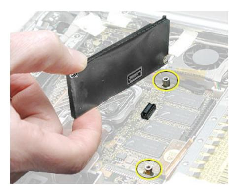
**Replacement Warning:** For the PowerBook G4 (12-inch DVI) model, make sure you reapply the transparent tape over the end of the modem so it overlaps the heatsink at the bottom of the fan, as shown.
