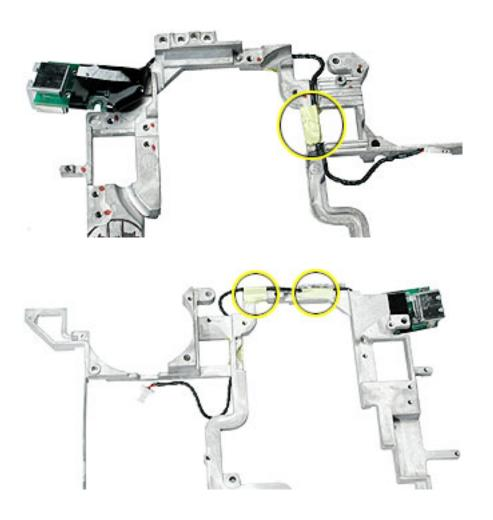
2. Remove the EMI shield from the RJ11 board. The board includes the attached cable and connector.
