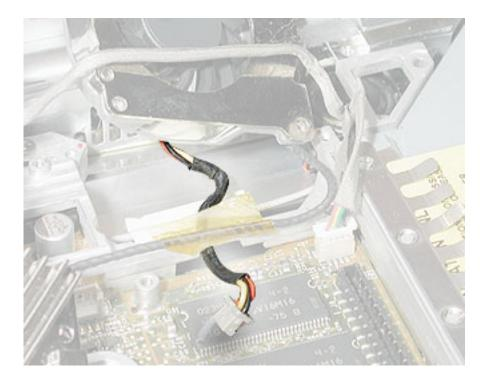
9. Note the routing of the remaining cables and the placement of tape once the heatsink is removed.
