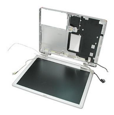
**Important:** The display might get caught on the hooks (shown below) on the bottom case. If so, gently twist the bottom case to release it from the display.
