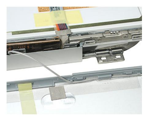
9. Install the replacement display housing, and reassemble and test the computer.
