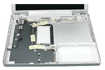
4. Note the routing of the AirPort antenna. Using a black stick, start to thread the AirPort antenna cable through the AirPort Extreme Card bay.
