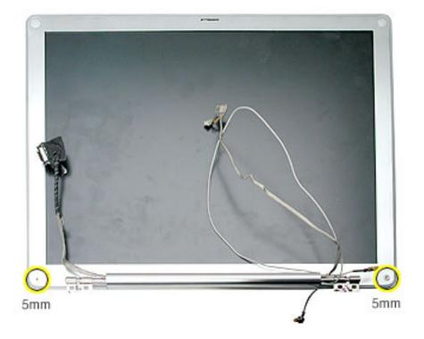
2. Use a black stick or thin plastic credit card around the outer edge of the bezel to separate the display housing tabs from the display assembly.
