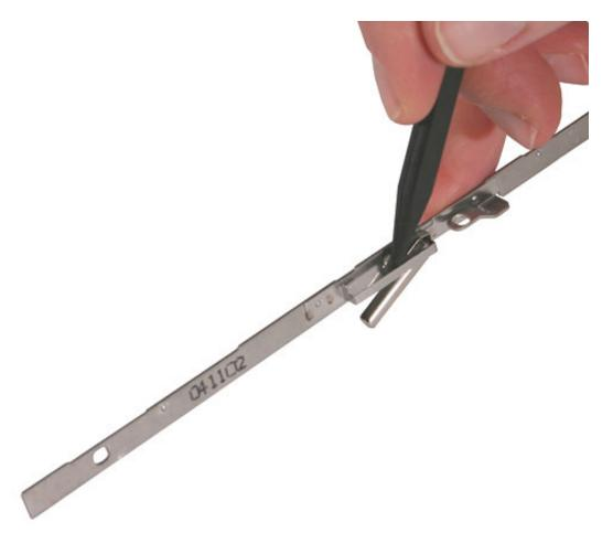
**Important:** Make sure the magnet is in place before reassembling the display module.
