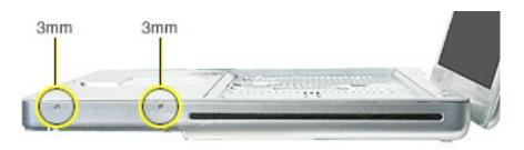
**Replacement Note:** In addition to securing the top case to the bottom case, the two 3-mm long screws help secure an inner bracket to the battery well. Make sure the bracket is installed in the bottom case before replacing the top case.
