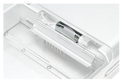
**Note:** The AirPort slot on the bottom case has a recessed inner slot designed for the clear plastic tab to tuck into.
