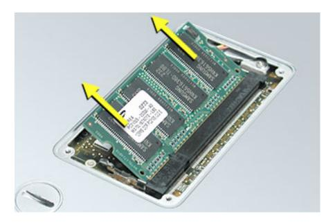
6. Insert the replacement memory card into the expansion slot at a 30-degree angle.
