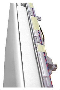
**Replacement Note:** Check that the orientation of the cables directed through the rear panel openings are as shown below:
