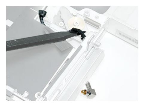
5. Holding the antenna cable near the strain relief, start to pull the antenna cable out through the corner of the card bay.
