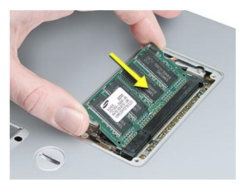
7. Make sure the memory card is fully inserted. Check that the notches in the card clear the tabs as you press down on the sides of the card to lock it into place.
