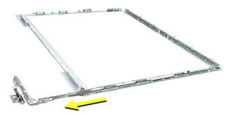
**Replacement Note:** To distinguish the right hinge with bezel brace from the left hinge with bezel brace, note that the right hinge has three flanges on the outer edge for the three screws. The left hinge has no screw flanges.
