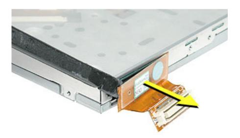
10. Install the replacement optical drive, and reassemble and test the computer.
