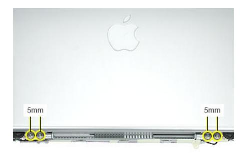
9. Remove the inner rear panel with attached speakers by routing the cables through the slots in the rear panel.
