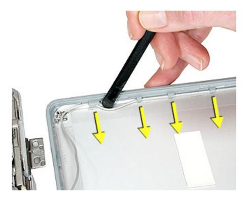
6. Move up the side of the display housing, releasing the cables from the tabs.
