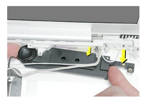
5. Install the replacement subwoofer, and reassemble and test the computer.
