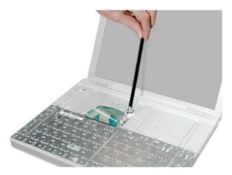
9. Peel up the keyboard cable from its adhesive. Using a black stick, pry up the tabs at the ends of the connector, and then pull the cable straight up to disconnect it.
