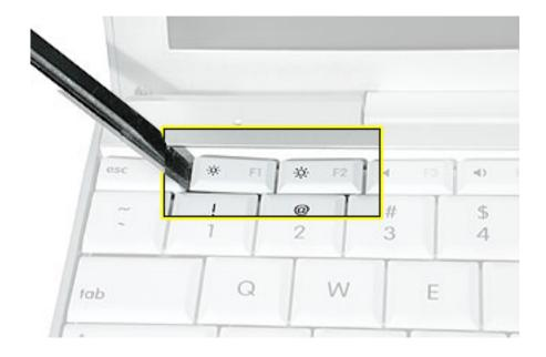
4. Use a black stick or flat-blade screwdriver to lift off the two round stickers that are located between the two key mechanisms. Reserve the stickers for replacement.
