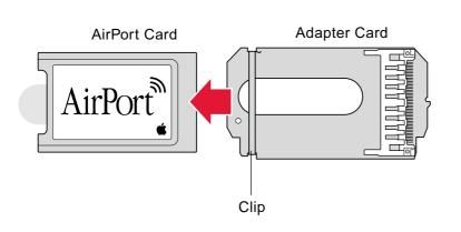
If an adapter card is installed on the AirPort card, release the metal clip and remove the AirPort card from the adapter.
