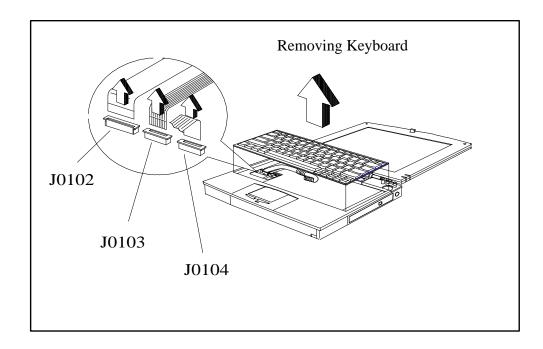
Figure 6-7 Removing/Replacing the Keyboard Assembly
