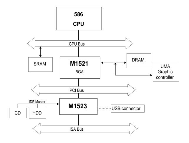
Figure 4-1 Extensa Functional Block Diagram
