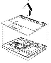
Figure 6-15 Removing/Replacing the Top Cover
