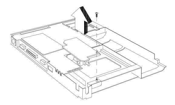
Figure 6-20 Removing/Replacing the Power Supply Board Assembly
