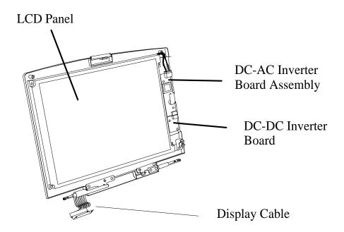
Display Assembly Shown with Bezel Removed
