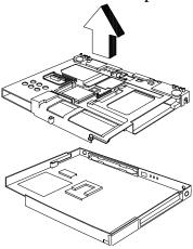
Figure 6-18 Detaching Base Assembly from Inside Frame Assembly
