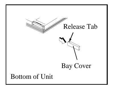
Figure 6-4 Removing the HDD Bay Cover
