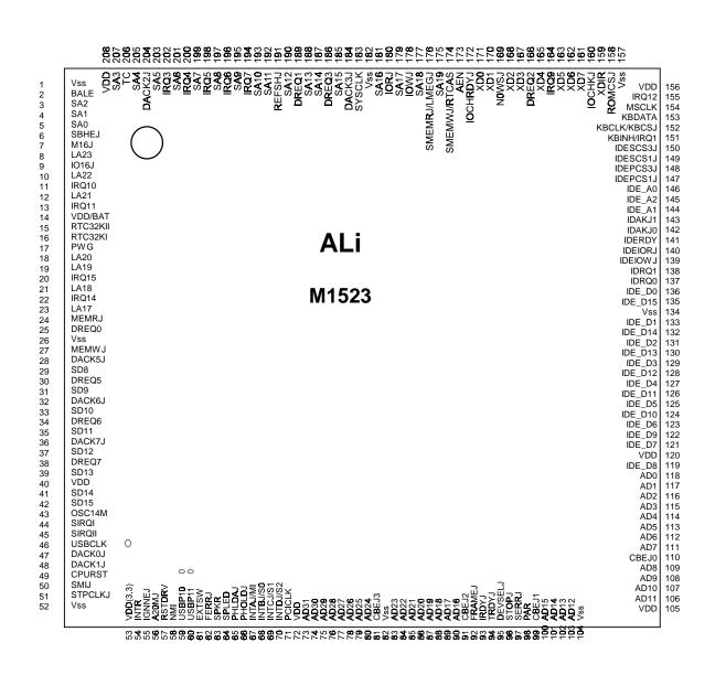
Figure 4-5 M1523 Pinouts
