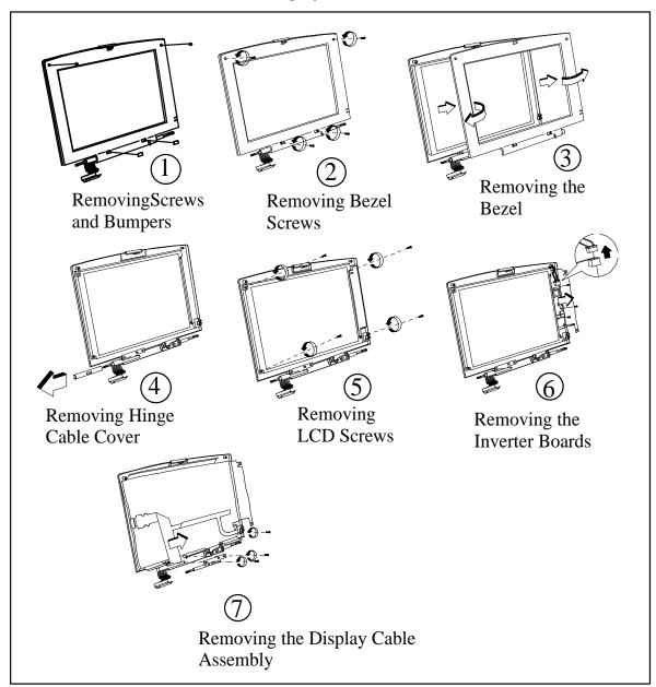
Figure 6-29 Display Unit Disassembly
