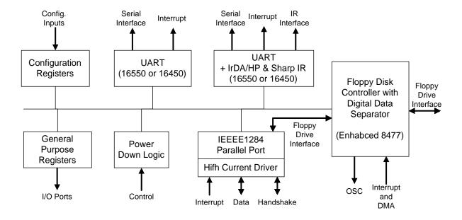
Figure 4-10 Super I/O Controller Block Diagram
