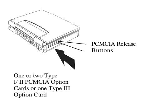
Figure 6-3 Installing/Removing PCMCIA Options
