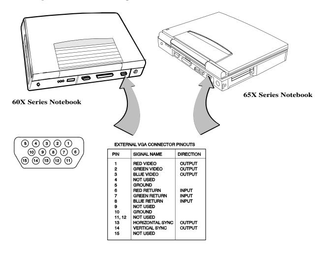
**Figure 2-7 External VGA Pinouts**
