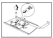
Remove two side screws and remove metal plate
