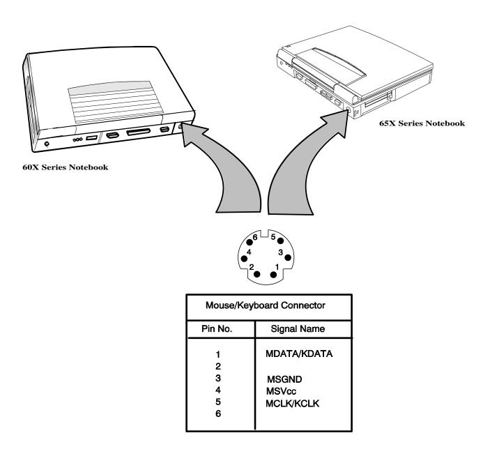
Figure 2-4 PS/2 Port Pinouts
