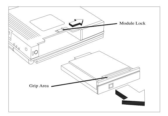
Figure 6-12 Removing/Replacing a 65x Series Module
