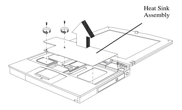
Figure 6-9 Removing/Replacing the Heat Sink Assembly
