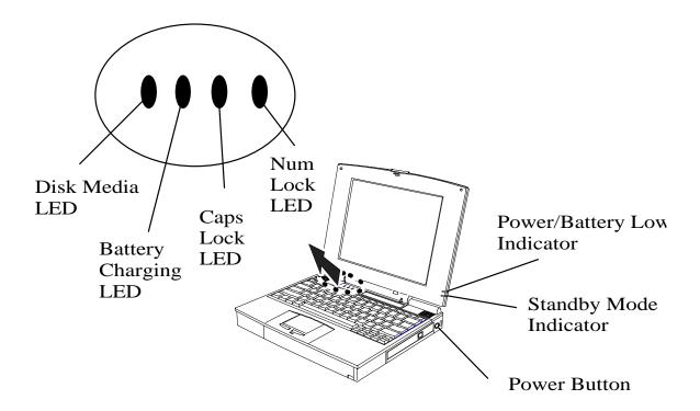
Figure 3-1 60x/65x Operating Controls and Indicators
