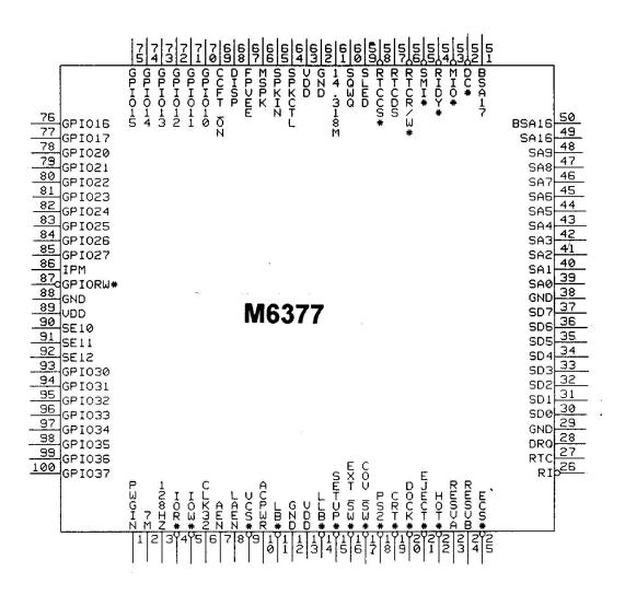
Figure 4-7 M6377 Chip Pinouts
