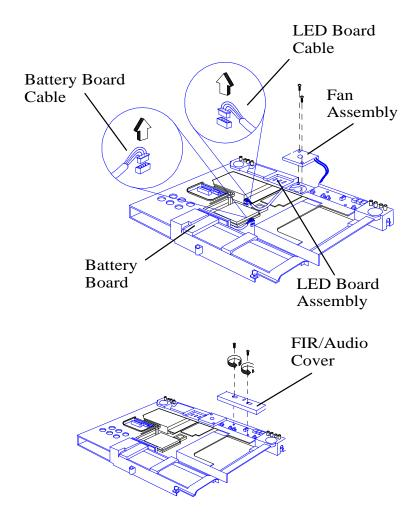
Figure 6-17 Internal PWB Assemblies, Removal/Replacement (65x Series)
