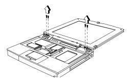
Figure 6-14 Removing the Display Hinge Screws
