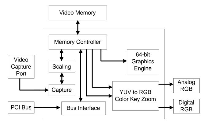
Figure 4-8 C&T65550 Simplified Block Diagram
