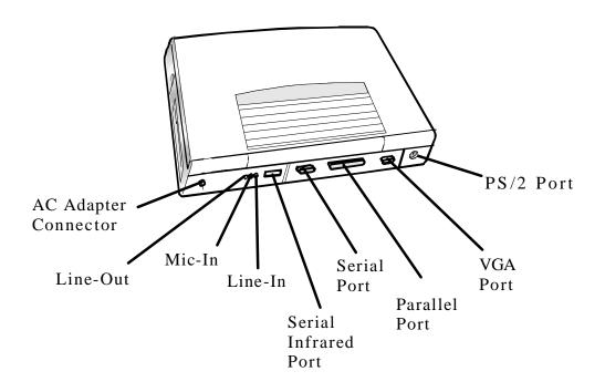
Figure 1-3 Extensa 60x External Ports
