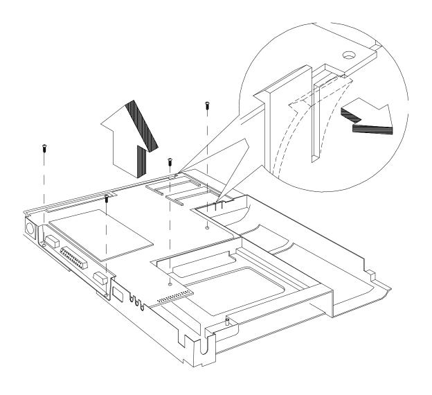
Figure 6-22 Detaching Motherboard from Inside Frame Assembly
