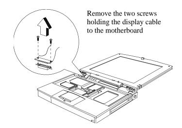
Figure 6-13 Unplugging the Display Cable
