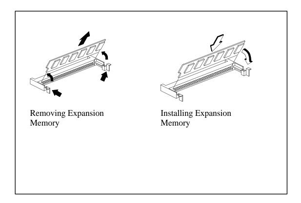
Figure 6-8 Memory Expansion Removal/Replacement
