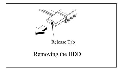
Figure 6-5 Removing/Replacing the Hard Disk Drive Module
