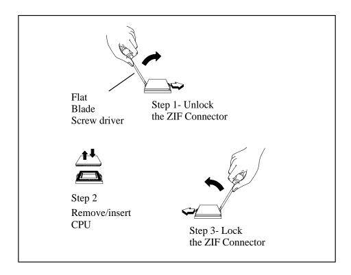
Figure 6-10 Removing/Replacing the CPU Chip
