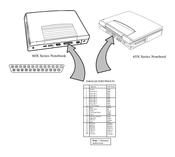
Figure 2-5 Parallel Port Pinouts
