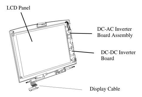
Display Assembly Shown with Bezel Removed
