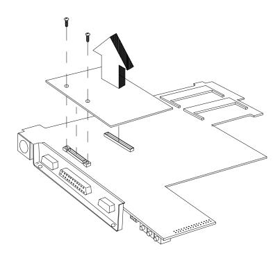
Figure 6-26 Removing/Replacing the VGA Video Board
