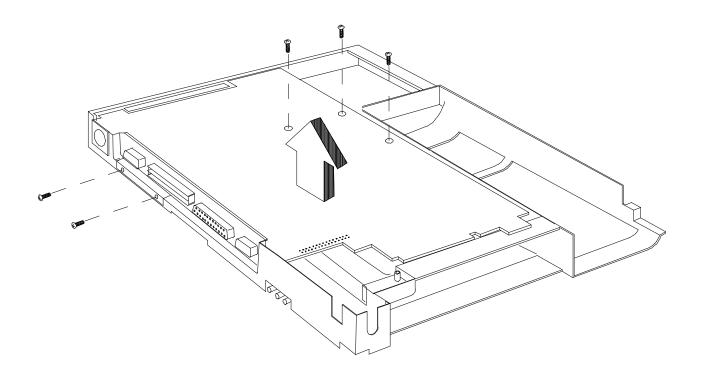
Figure 6-23 Detaching Motherboard from Inside Frame Assembly
