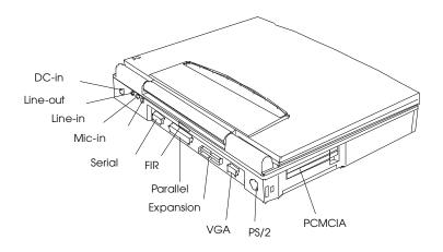
Figure 1-4 65x Series External Ports
