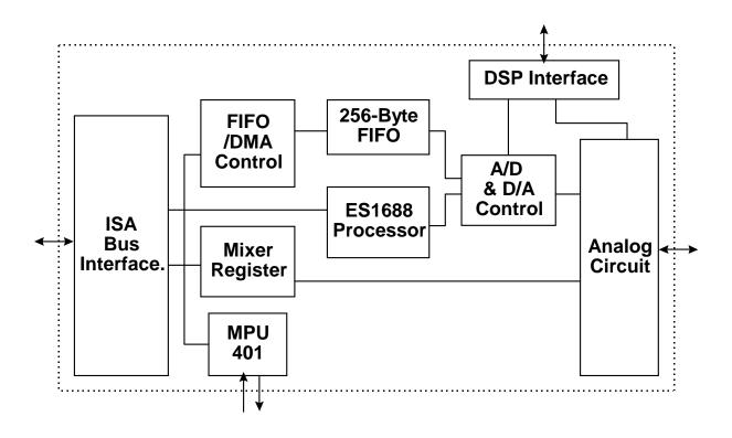
Figure 4-11 ES1688 Sound Chip Block Diagram
