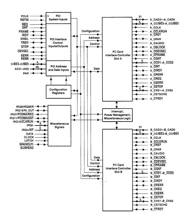
Figure 4-9 PCMCIA Controller, Simplified Block Diagram
