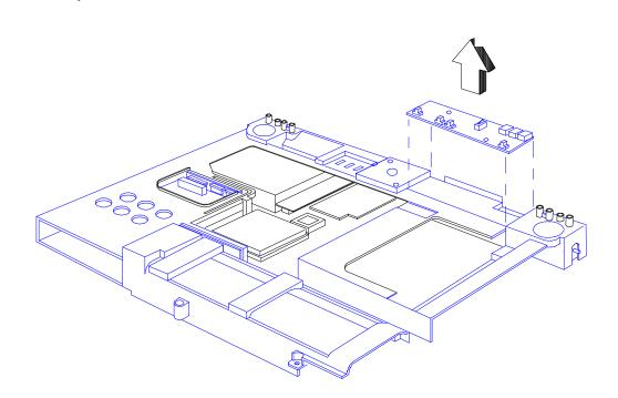
Figure 6-24 Removing/Replacing the FIR/Audio Board
