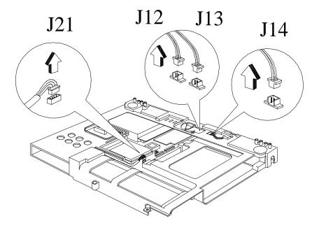
Figure 6-21 Unplugging Cables on 60x Series Motherboard
