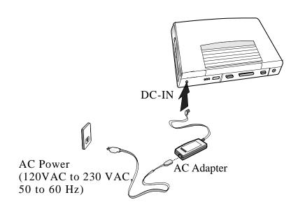
Figure 2-12 - Installing the AC Adapter
