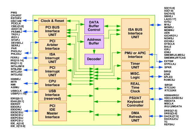
Figure 4-4 M1523 Chip Simplified Block Diagram
