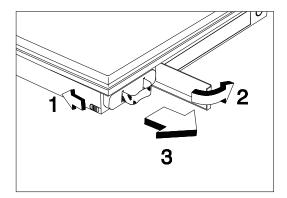
Figure 2-3 Battery Pack Installation
