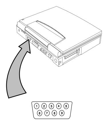
Figure 2-6 Serial Port Pinouts
