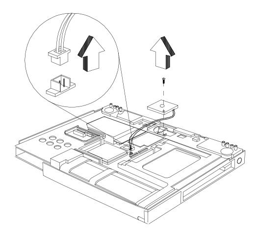
Figure 6-16 Removing/Replacing the Fan Assembly (60x Series)
