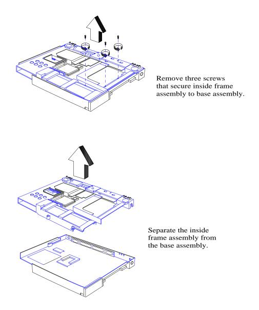
Figure 6-19 Removing/Replacing the Inside Frame Assembly (65x Series)
