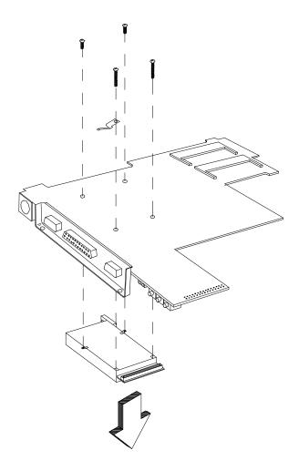
Figure 6-26 Removing/Replacing the PCMCIA Module
