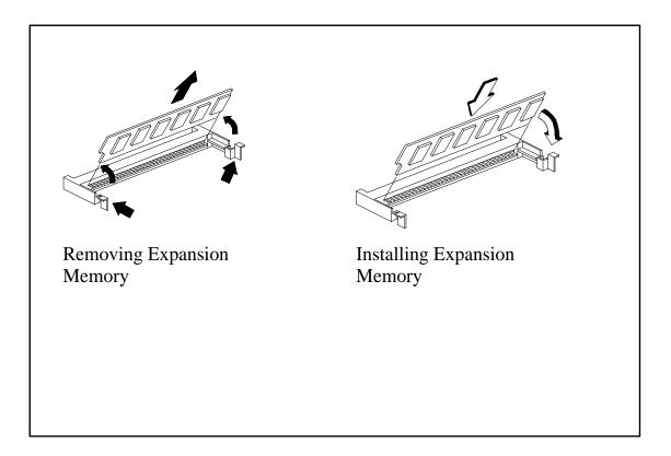
Figure 2-1 Memory Expansion Removal/Replacement
