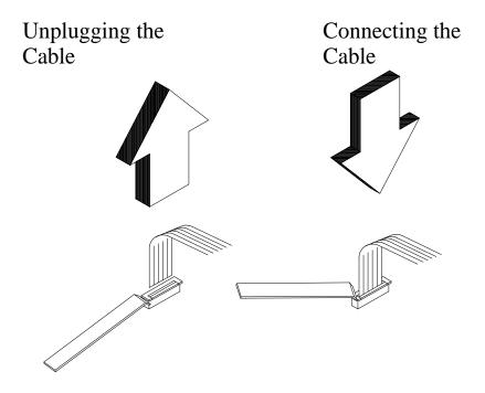
Figure 6-1 Removing/Installing Cables with Locking-Type Connectors
