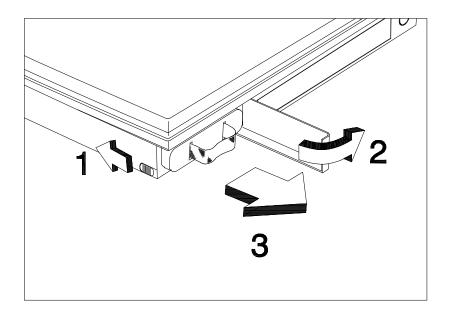
Figure 6-2. Battery Removal/Replacement
