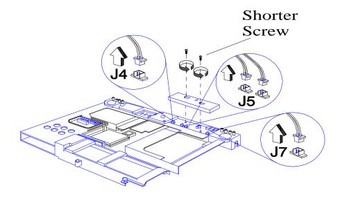
Figure 6-24 Unplugging Cables on Motherboard (65x Series)
