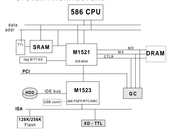
Figure 4-2 Extensa Series System Architecture Diagram
