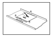
Figure 6-28 Removing/Replacing the Touchpad Assembly
