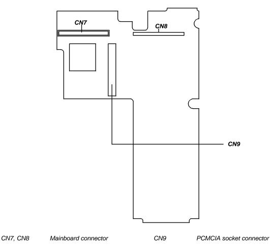
*Figure 1-12 Media Board Jumpers and Connectors (Bottom Side)*
