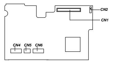
CN2Lid switchCN6Touchpad connectorCN1LCD connectorCN4, CN5Keyboard connector
