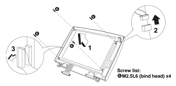
Figure 4-28 Removing the Display Panel Screws and the Display Connectors
