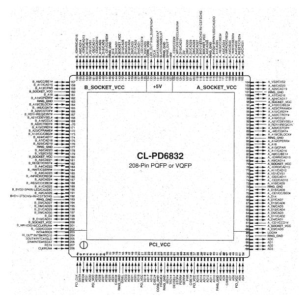
Figure 2-10 CL-PD6832 Pin Diagram
