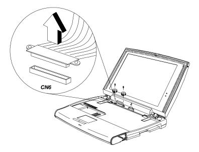
Figure 4-15 Unplugging the Display Cable
