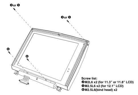
3. Pull out and remove the display bezel by pulling on the inside of the bezel sides.
