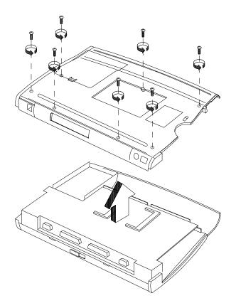
Figure 4-17 Removing the Lower Housing
