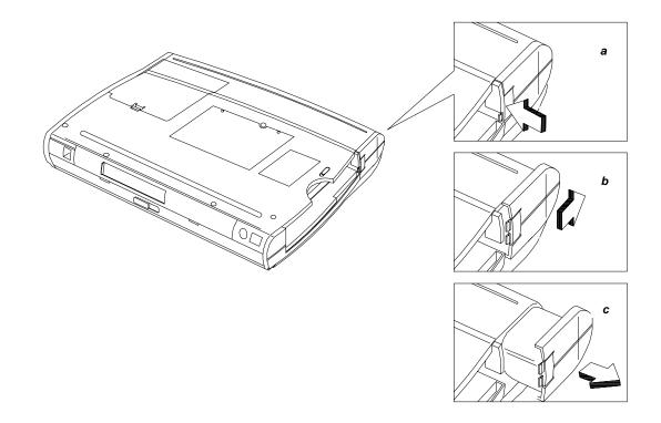
Figure 4-1 Removing the Battery Pack
