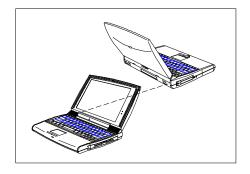
To use the infrared port, position two IR-aware devices such that their IR ports are no more than one meter apart and offset no more than 15 degrees.
