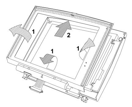
Figure 4-27 Removing the Display Bezel
