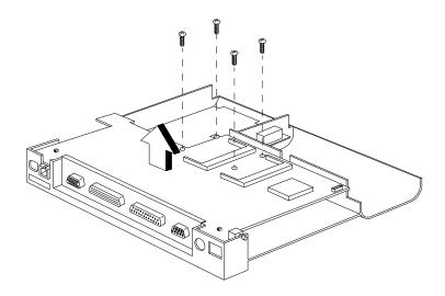
Figure 4-22 Removing the Main Board
