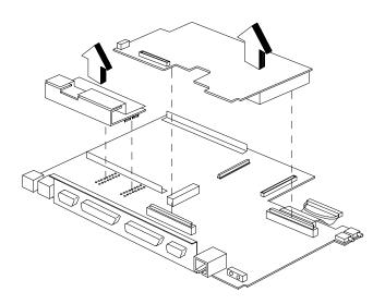
Figure 4-23 Removing the Charger Board and Multimedia Board
