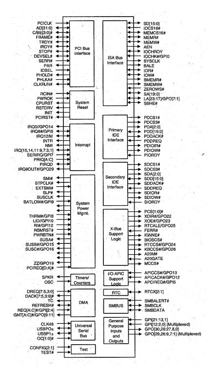
Figure 2-2 PIIX4 Simplified Block Diagram
