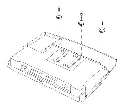
Figure 4-18 Removing the Battery Bay Screws
