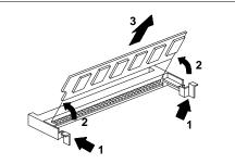
Figure 4-8 Installing and Removing Memory
