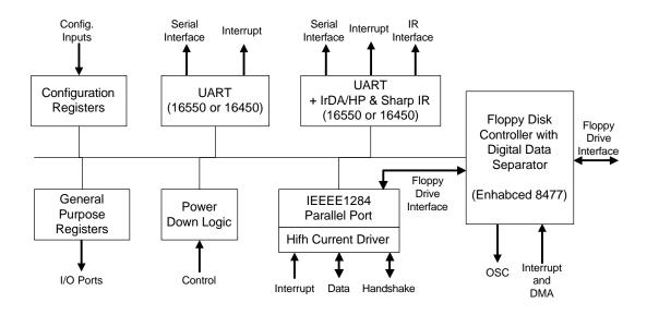
Figure 2-8 NS87338VJG Block Diagram
