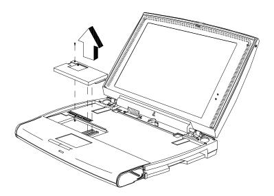
Figure 4-14 Removing the CPU Module
