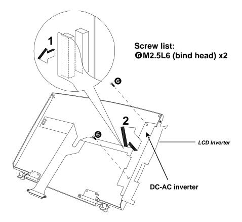
Figure 4-29 Removing the Display Cable Assembly
