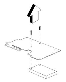
Figure 4-24 Removing the PC Card Slots
