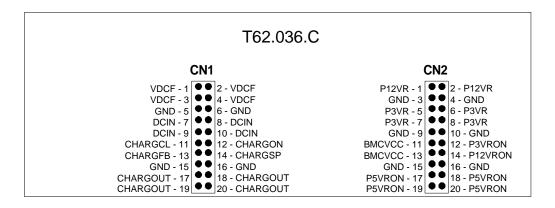
Figure 2-11 T62.036.C Pin Diagram
