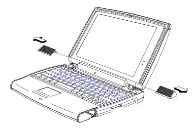
Figure 4-9 Removing the Display Hinge Covers
