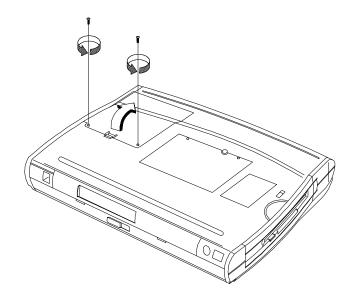
Figure 4-5 Removing the Hard Disk Drive Bay Cover
