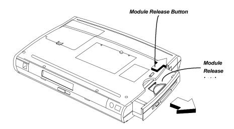
Figure 4-4 Removing the Module
