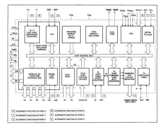
Figure 2-6 87C552 Block Diagram
