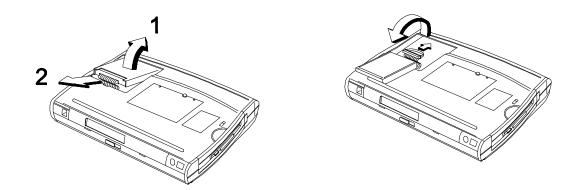
Figure 4-6 Removing the Hard Disk Drive
