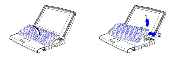
Figure 4-11 Lifting Out the Keyboard
