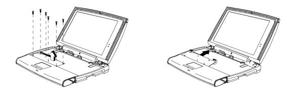
Figure 4-13 Removing the CPU Heat Sink
