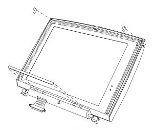
Figure 4-25 Removing the LCD Bumpers
