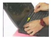
3. Remove the middle hinge cap from the main unit.
