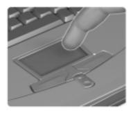
**NOTE:** When using an external USB or serial mouse, you can press Fn + [7] to disable the touchpad. If you are using an external PS/2 mouse, the touchpad is automatically disabled.
