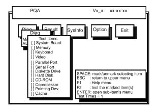
Move the highlight bar from one item to another. Press Space to enable or disable the item. Press e to view the available options of each selected item. Press | to close the submenu.
