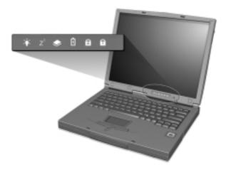
The Power and Standby status icons are visible even when you close the display cover so you can see the status of the computer while the cover is closed.
