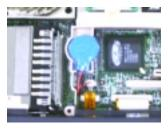
4. Remove the RTC battery.
