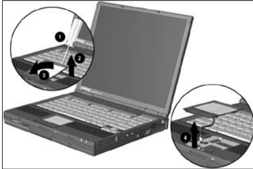
Figure 5-6. Removing the Touch Button
