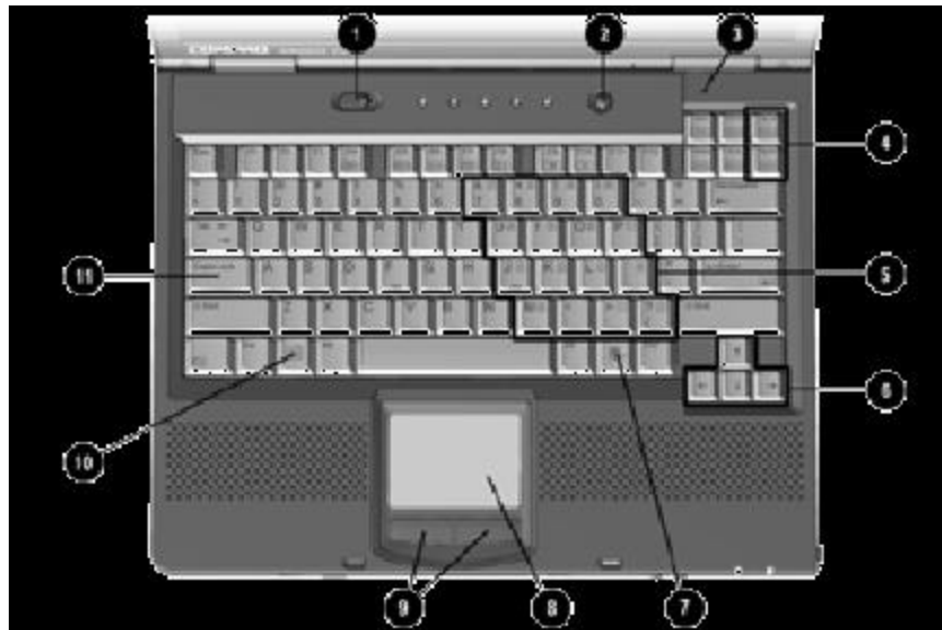
Figure 1-5. Keyboard Components
