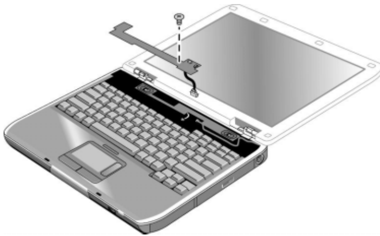
Figure 2-13. Removing the Switchboard PCA HP Pavilion 4300, 4200, and 4100, HP nx9005 and nx9000, Compaq Evo Notebook N1050 and 1010, and Compaq Presario 2100 and 1100 Models
