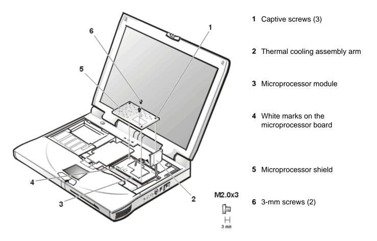
To remove the microprocessor module, perform the following steps.
