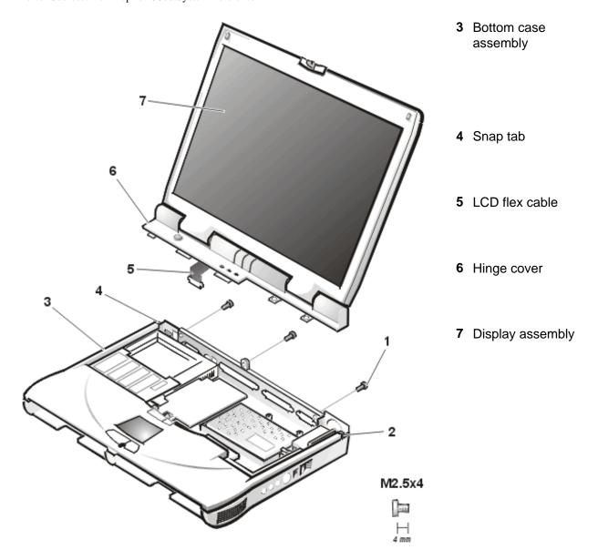
To remove the display assembly, perform the following steps.
