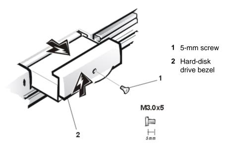
To remove the hard-disk drive assembly, perform the following steps.
