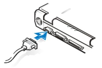
Be sure to tighten all the screws on the video cable connector(s) to eliminate radio frequency interference (RFI).
