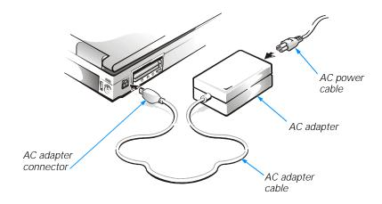
Figure 2-1. Using the AC Adapter
