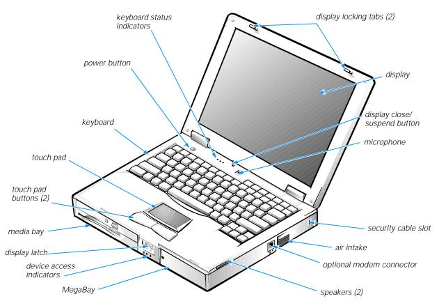
Figure 1-1. Front View of the Computer
