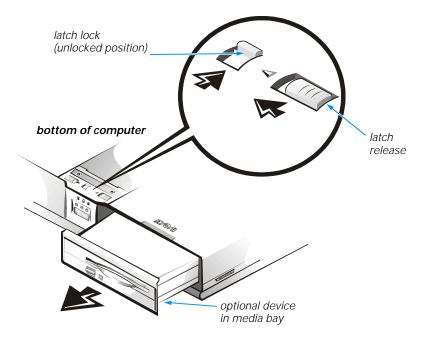
Figure 2-2. Removing a Device From the Media Bay
