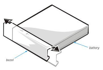
Figure 2-4. Adjusting the Battery Bezel
