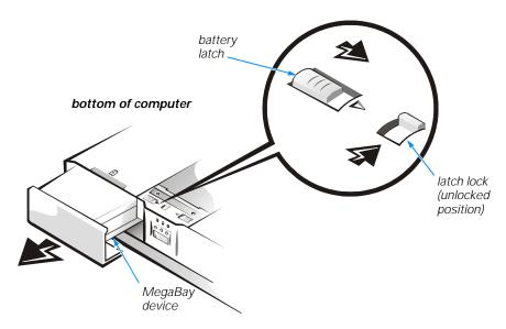
Figure 2-3. Removing a Device From the MegaBay
