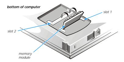
Figure 2-9. Removing a Memory Module
