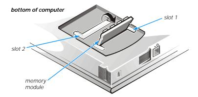
Figure 2-10. Installing a Memory Module
