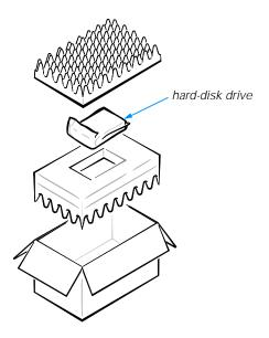
Figure 2-7. Repackaging the Hard-Disk Drive
