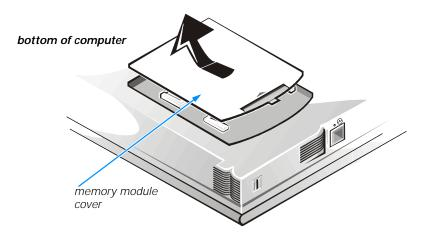
Figure 2-8. Removing the Memory Module Cover
