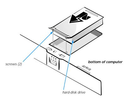
Figure 2-6. Removing the Internal Hard-Disk Drive
