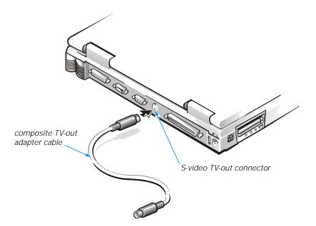
Figure 2-5. Using the Composite TV-Out Adapter Cable
