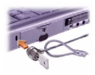
The slots (one on each side of the computer) let you attach a commercially available antitheft device to the computer. Complete instructions for installing antitheft devices are usually included with the device.
