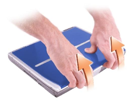
2. Firmly grasp the lip of the cover to detach it from the computer, and pull the cover up.
