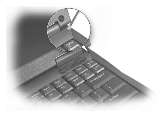
5. To release the keyboard from the palm rest, use a small, flat-blade screwdriver or plastic scribe to pry up the right edge of the keyboard near the blank key.
