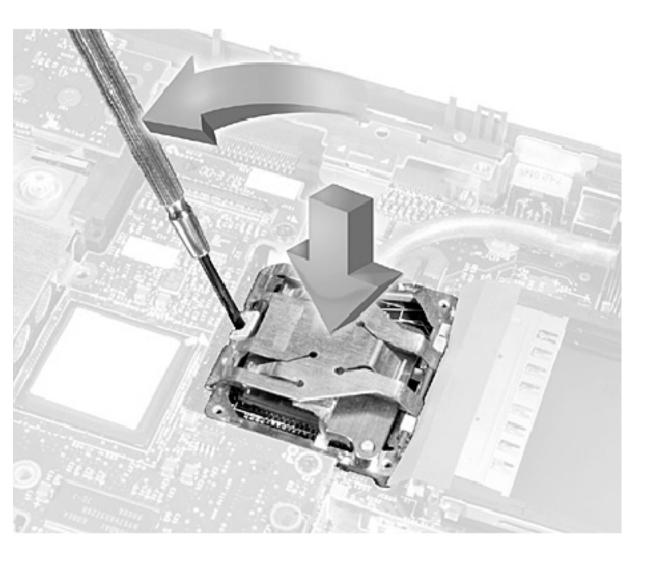
4. While pressing lightly down on the center of the retaining clip, insert a flat-blade
