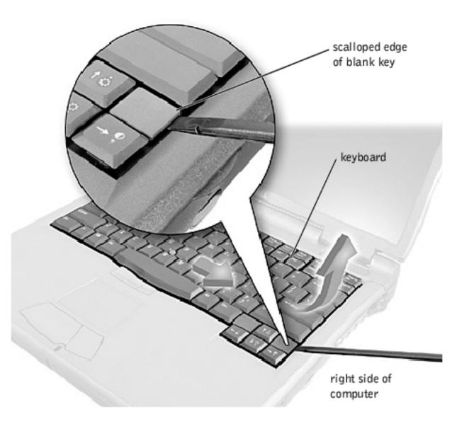
5. Lift the right end of the keyboard and slide it slightly toward the right side of the computer to disengage the tabs at the left end.
