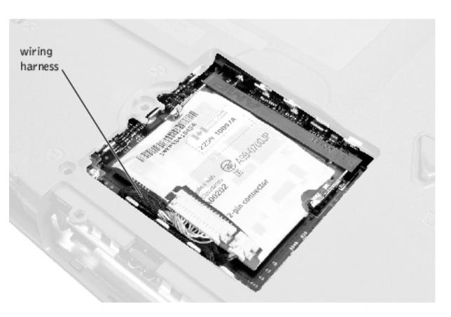
**Mini-PCI Wireless NIC Assembly Using Antenna Cable**
