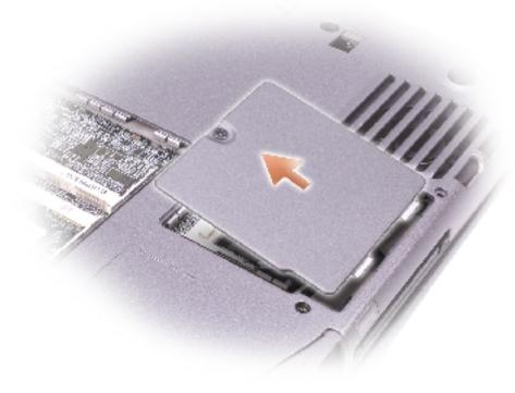
3. Place your finger under the cover at the indentation, lift up the cover, and slide the cover open.
