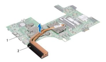
1 captive screws (6) 2 thermal cooling assembly
