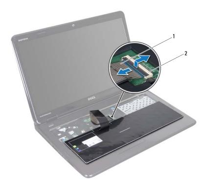
1 keyboard cable 2 keyboard-cable connector
