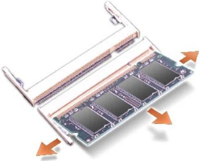
➡ **NOTICE:** If you need to install memory modules in two connectors, install a memory module in the connector labeled "JDIM (Slot 1)" before you install a module in the connector labeled "JDIM2."
