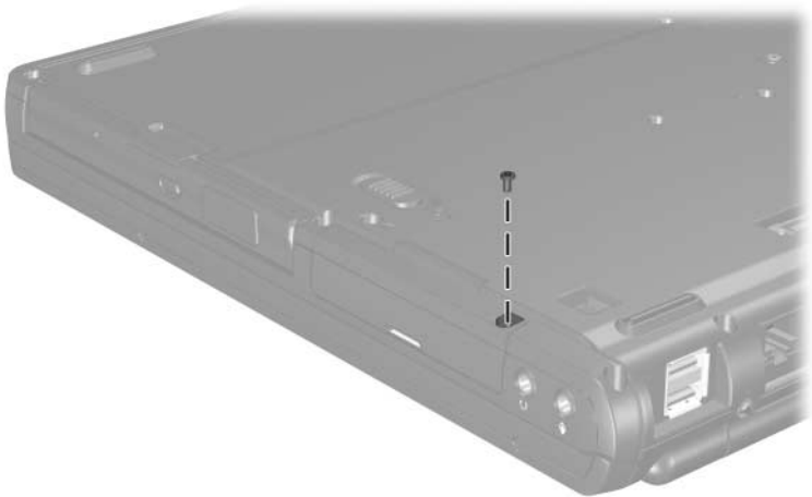
Phillips PM2.0x4.0 Hard Drive Cover Screw Location
