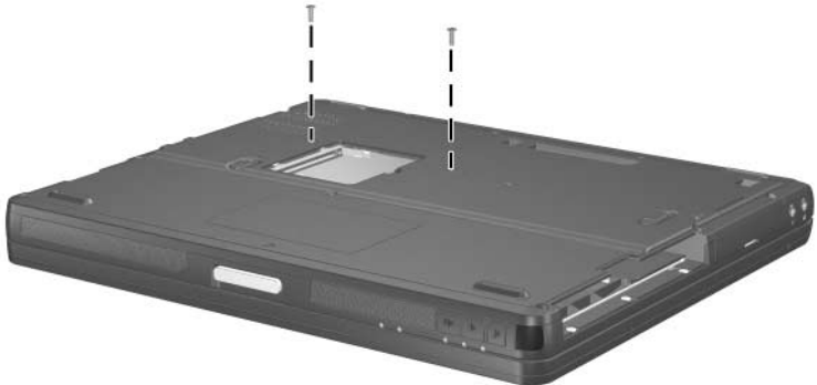
Torx T8M2.5×9.0 Keyboard Access Screw Locations
