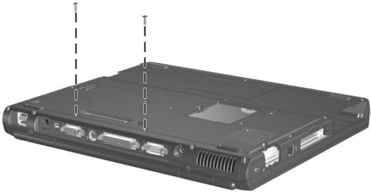
Torx T8M2.5×9.0 Switch Cover Screw Locations
