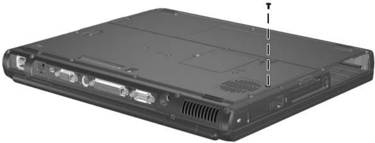
Torx T8M2.5x5.0 Fan Assembly Screw Location
