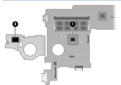
**NOTE:** The following illustration shows the replacement thermal material locations. Thermal paste is used on the processor (1) and the heat sink section (2) that services it.
