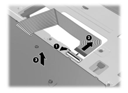
Reverse this procedure to install the keyboard.
