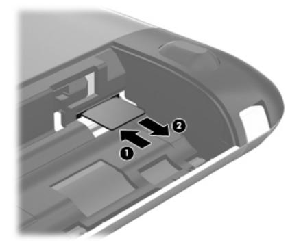
Insert the SIM into the SIM slot, and gently push the SIM into the slot until it is firmly seated.
