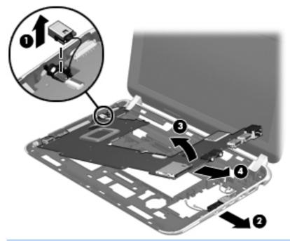
**NOTE:** If it is necessary to replace the power connector cable, turn the system board upside down with the rear toward you, and then disconnect the power connector cable from the system board. The power connector cable is available using spare part number 656095-001.
