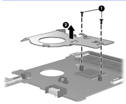
The thermal material must be thoroughly cleaned from the surfaces of the heat sink and the system board components each time the heat sink is removed. Replacement thermal material is included with the heat sink and system board spare part kits.
