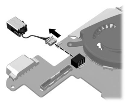
Reverse this procedure to install the system board and the power connector cable.
