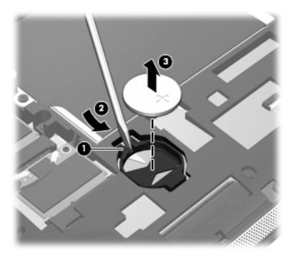
Reverse this procedure to install the RTC battery. When installing the RTC battery, be sure the "+" sign faces up.
