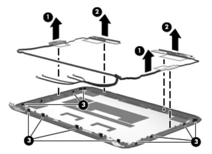
c. Remove the wireless antenna cables and transceivers. The wireless antenna cables and transceivers are available in the Antenna Kit, spare part number 658498-001.
