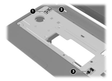
**14.** Remove the five Phillips PM2.0×5.0 screws that secure the top cover to the base enclosure.
