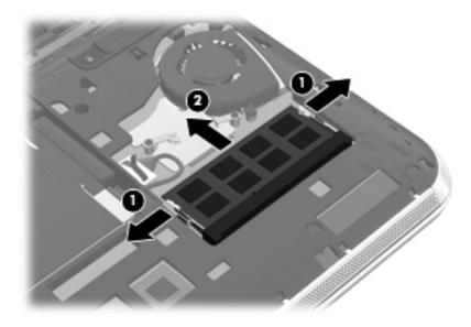
Reverse this procedure to install the memory module.
