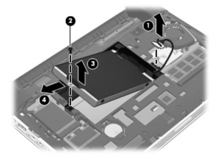
5. If it is necessary to replace the hard drive connector cable (1), the hard drive screws (2), the hard drive bracket (3), or the rubber isolators (4), remove and replace the components.
